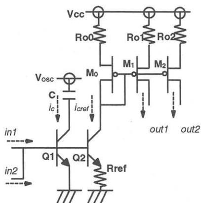
Fig. 7. Proposed application of capacitance-npn-transistor circuit to a neuron element.
