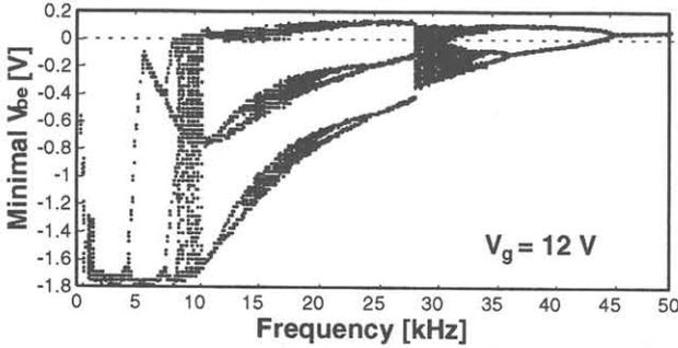
Fig. 4. Measured bifurcation diagram
