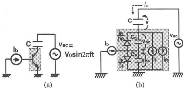
**Fig. 1.** (a) Fundamental circuit of capacitance-npn-transistor circuit. (b) Equivalent circuit which includes parasitic capacitance in the npn transistor.
