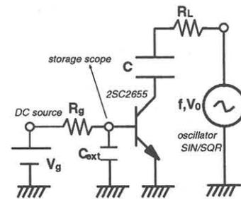
**Fig. 2.** Experimental circuit. NPN transistor is type 2SC2655,  $C = 4.7\text{nF}$ ,  $R_g = 1\text{M}\Omega$ ,  $R_L = 1\text{k}\Omega$  and  $C_{ext} = 680\text{pF}$
