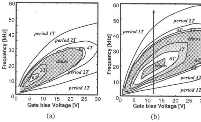
Fig. 3. Measured parameter region ( $V_g, f$ ) in which the system results in period-multiplying / chaotic states, (a) under sinusoidal- and (b) square-wave excitation.
