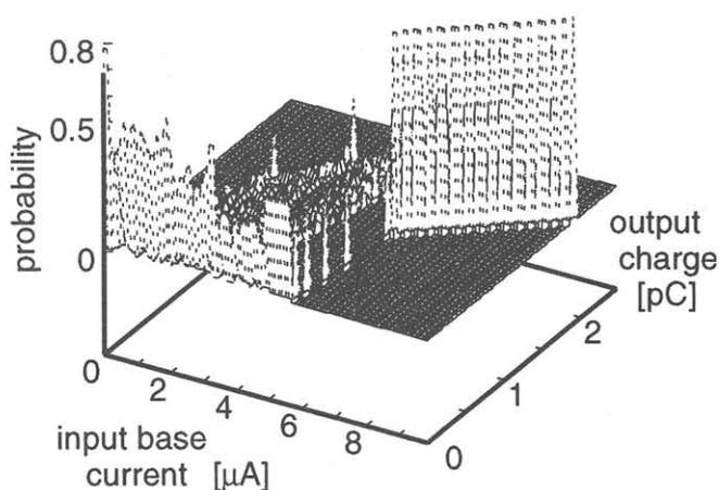
Fig. 9. Histogram of output charge according to input current.
