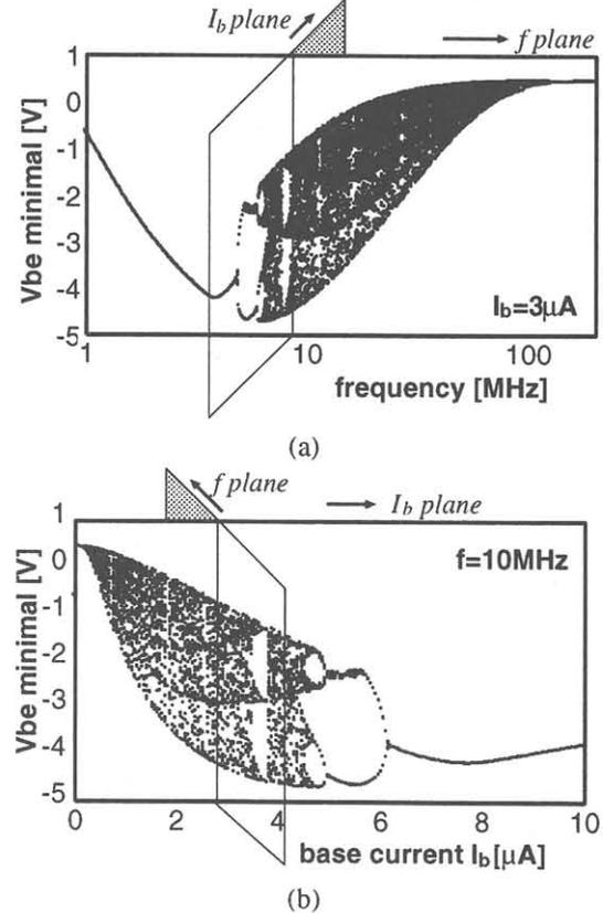
Fig. 6. Simulated bifurcation diagram of minimal  $v_{be}$  according to (a)  $f$  with  $I_b = 3\mu\text{A}$  and (b)  $I_b$  with  $f = 10\text{MHz}$ .
