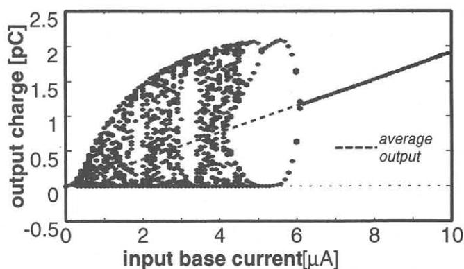
Fig. 8. Net charge of  $i_{cref}$  in a positive half cycle according to input current. Dashed line in the schematic expresses the average of the output charge.
