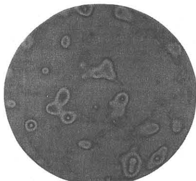
Fig. 3 Photograph of SiO 2 -deposited wafer after 5 min-CMP using the vacuum chuck. The fringes correspond to the local thickness fluctuations of the SiO 2 film. During CMP, abrasive silica particles in the slurry were aspirated and dried on the wafer reverse or the chuck surfaces, resulting in local wafer deformations and polishing defects.
