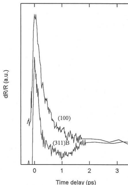
Fig. 1 Transient reflectivity of as-grown LT-GaAs layer grown on (100) and (311)B GaAs substrates.
