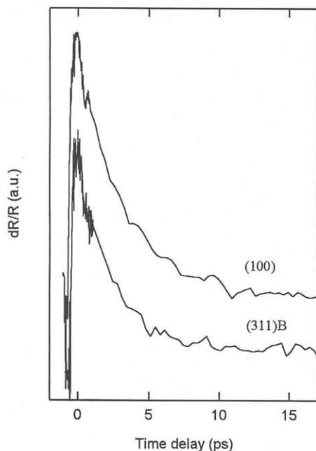
Fig. 2 Transient reflectivity of 600 °C annealed LT-GaAs layer grown on (100) and (311)B GaAs substrates.
