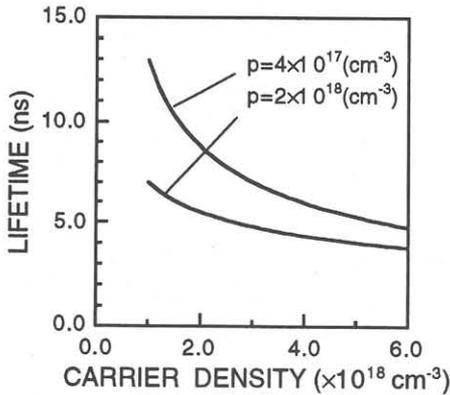
Fig. 1. Relationship between carrier lifetime and optically pumped carrier density in the saturable absorbing layer.
