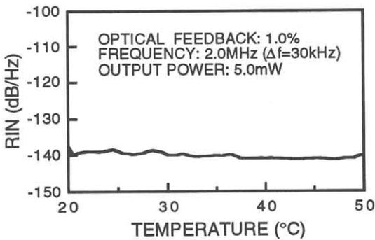
Fig. 4. Temperature dependence of the relative intensity noise (RIN) at the output power of 5.0 mW. Low noise characteristics was realized in the high temperature range as well as low range.
