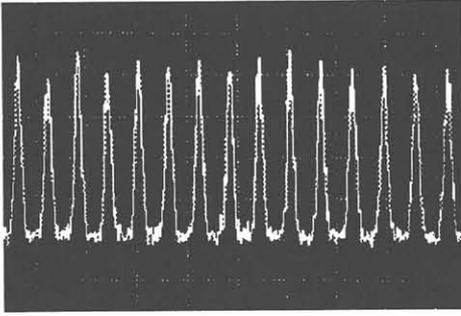
Fig. 3. Time dependence of the output power measured by using an optical oscilloscope at an average power of 5 mW. The continued oscillation with a frequency of 0.82GHz was confirmed. (Horizontal: 2ns/div.)
