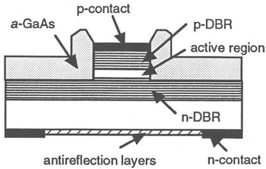
Figure 1. Schematic diagram of amorphous-GaAs-buried surface-emitting lasers.
