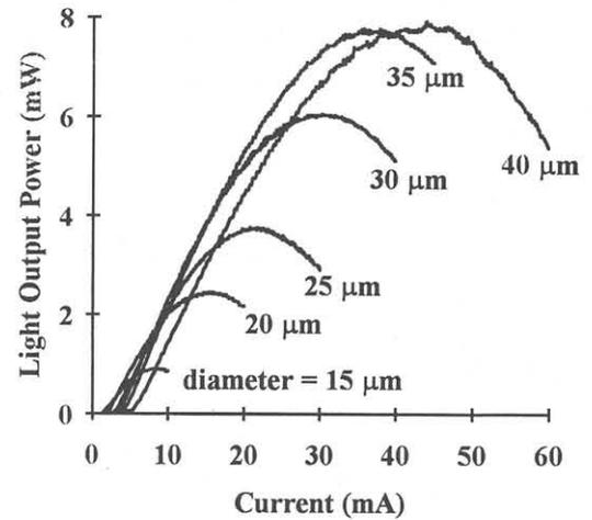
Figure 2. CW light output against current characteristics for amorphous-GaAs-buried lasers.
