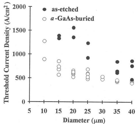
Figure 3. Threshold current densities for air-post and amorphous-GaAs-buried lasers.
