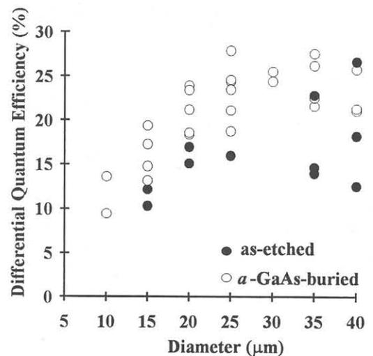
Figure 4. Differential quantum efficiencies for air-post and amorphous-GaAs-buried lasers.
