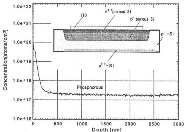
Figure 3. Depth profile of phosphorous obtained with SIMS for a pn homo-junction. Schematic depiction of the light emitting pn junction diode is also shown.
