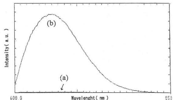
**Figure 1.** Photoluminescence spectra from (a) as-doped and (b) after electrical etching at room temperature.
