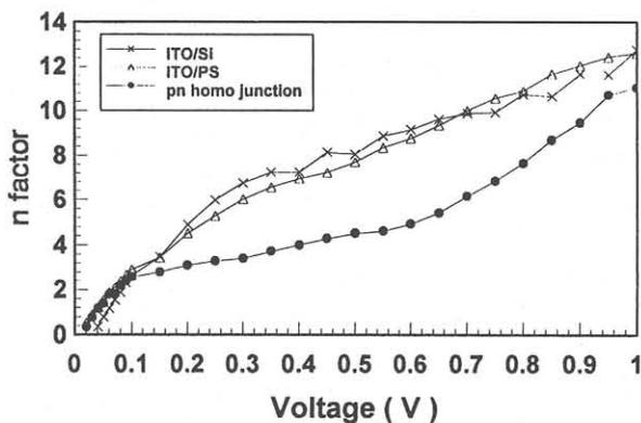
Figure 5. Forward voltage dependence of ideal  $n$  factor.
