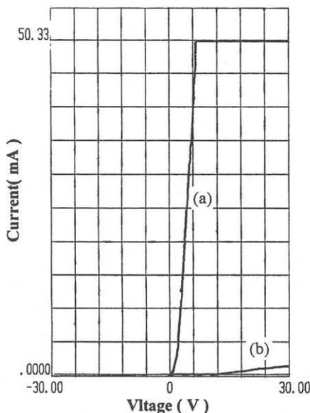
Figure 4. I-V characteristics of (a) a pn homo-junction diode and (b) a Schottky diode at room temperature.
