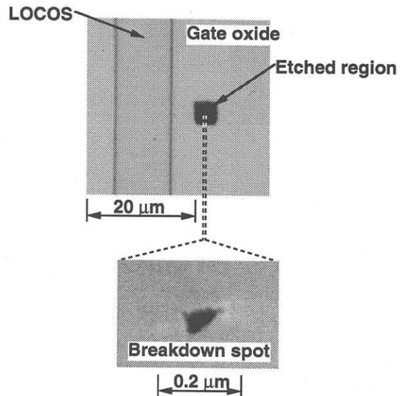
Fig. 2. Photographs from optical microscopy image (top) and SEM image (bottom) after Cl-radical etching of MOS diode with 6 nm gate oxide.
