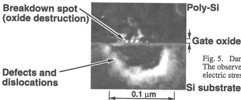
Fig. 5. Dark field image of cross-sectional TEM. The observed sample was MOS diode with appeared electric stress of -9 V.
