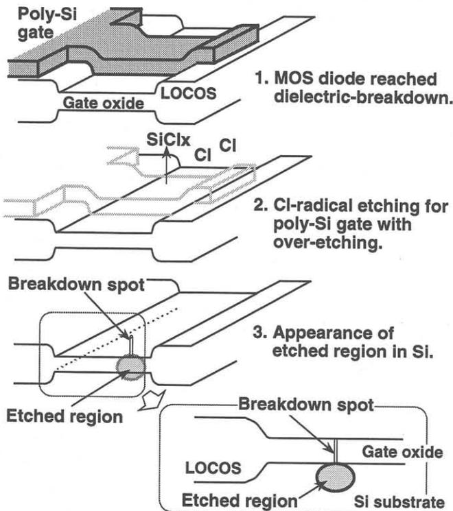
Fig. 1. The process to identify the breakdown spot of a MOS diode by high-selectivity Cl-radical etching.
