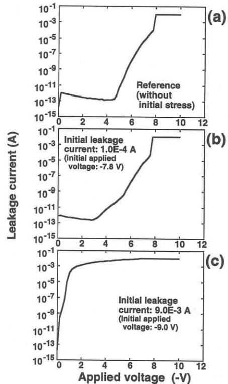
Fig. 4. I-V characteristics of MOS diodes. The initial stress was applied prior to I-V measurement. (a) Reference sample without stress, (b) not reaching dielectric-breakdown, and (c) resultant initial-short by intrinsic breakdown.
