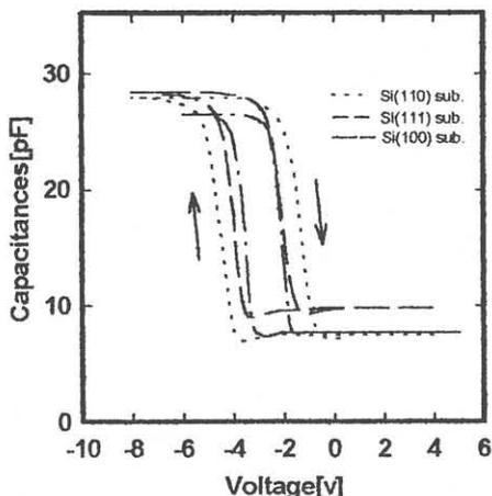
Fig. 2. 1 MHz C-V characteristics of MFS capacitors fabricated on Si(100), (110) and (111) oriented substrates, respectively.
