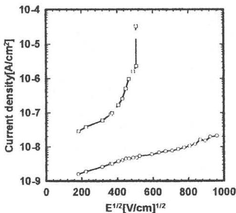
Fig. 1. I-V characteristics denoted by current density and square root of electric field of MFS capacitors biased at accumulation state.
