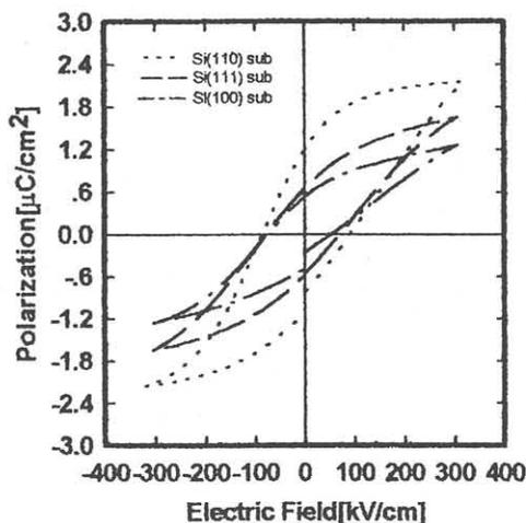
Fig. 3. Polarization hysteresis loop of MFS capacitors fabricated on Si(100), (110) and (111) oriented substrates.
