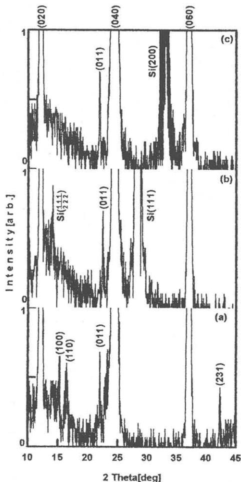
Fig. 4. XRD patterns of the  $\text{BaMgF}_4$  films on (a) Si(110), (b) Si(111) and (c) Si(100) oriented substrates.
