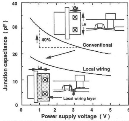
Fig. 1 Junction capacitance per inverter as a function of power supply voltage.  $W_a=1.5\mu\text{m}$ ,  $L_a=6\mu\text{m}$  for conventional structure,  $W_a=0.5\mu\text{m}$ ,  $L_a=6\mu\text{m}$  for local wiring structure.
