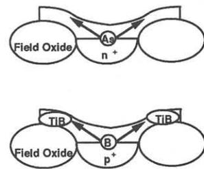
Fig. 5 Illustration of dopant-redistribution. 1st stage illustrates diffusion of dopant from Si to  $\text{TiSi}_2$ , 2nd stage  $\text{TiSi}_2$  to Si.
