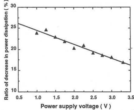
Fig. 7 Ratio of decrease in power dissipation applying local wiring as a function of power supply voltage. Power dissipation is measured by 101 stages ring oscillator. Gate length is  $0.35\mu\text{m}$ , active width is  $1.8\mu\text{m}$  for conventional,  $0.4\mu\text{m}$  for local wiring structure.
