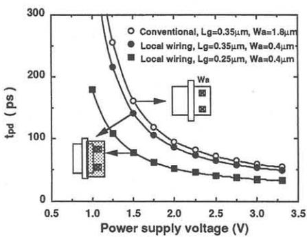
Fig. 6 Propagation delay time as a function of power supply voltage measured by 101 stages ring oscillator.
