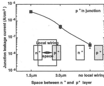
Fig. 3 Junction leakage current with  $n^+$  and  $p^+$  layer by  $\text{TiSi}_2$  local wiring. Leakage current is measured at reverse bias of 3.3V
