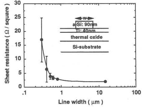
Fig. 2 Sheet resistance of  $\text{TiSi}_2$  film as a function of line width
