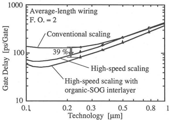
Fig. 7. Calculated gate delay from measured wiring capacitance and resistance.
