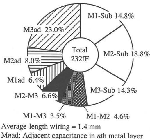
Fig. 1. Wiring capacitance components extracted from 0.5- $\mu\text{m}$  ASIC gate arrays.
