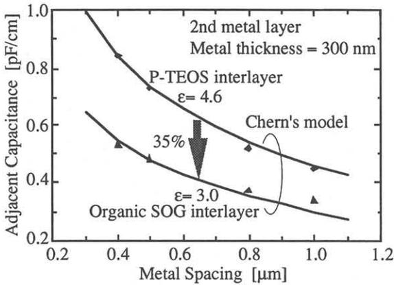
Fig. 6. Measured adjacent capacitance as a function of metal spacing.
