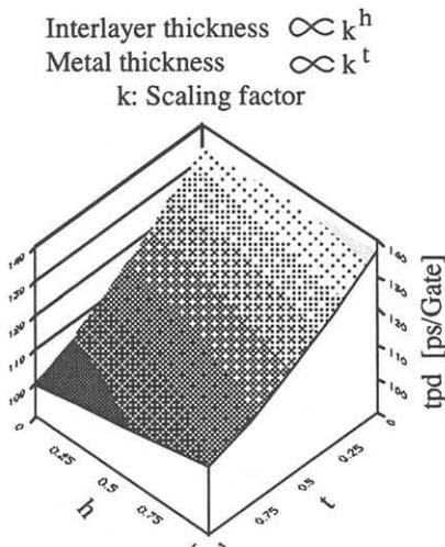
Fig. 3. Dependence of gate delay on scaling parameters  $h$  and  $t$  after scaling down to 0.25- $\mu\text{m}$ .
