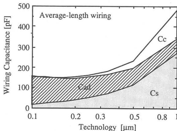
Fig. 2. Dependence of the wiring capacitance component on fabrication technology in average-length wiring.
