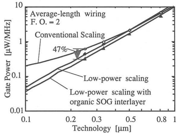
Fig. 8. Calculated gate power from measured wiring capacitance and resistance.
