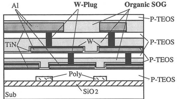
Fig. 4. Schematic cross section of a fabricated interconnect structure for a 0.25- $\mu\text{m}$  ASIC.
