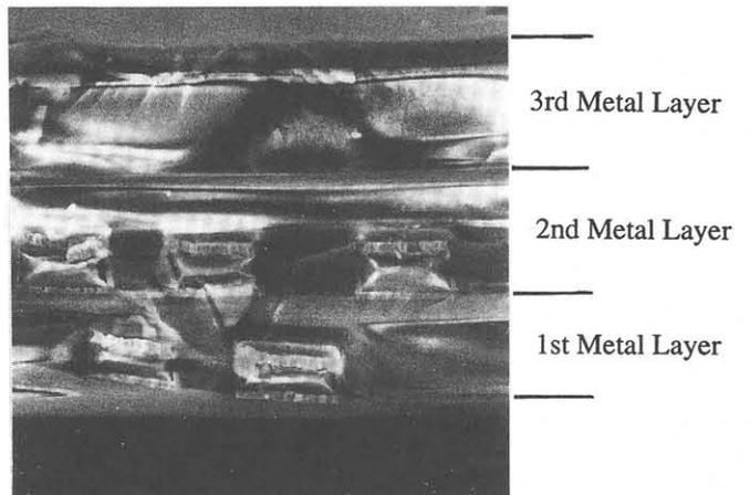
Fig. 5. SEM photograph of a cross section of the fabricated interconnect structure.
