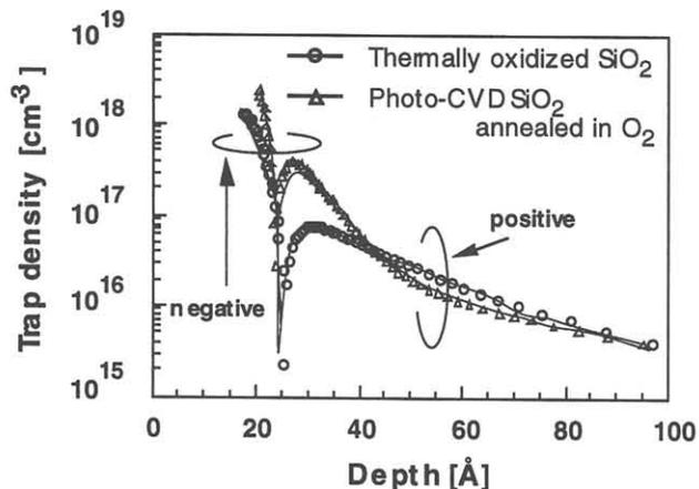
Fig. 4. Spatial distributions of the photo-CVD SiO<sub>2</sub> film annealed in O<sub>2</sub> and the thermally oxidized SiO<sub>2</sub> film
