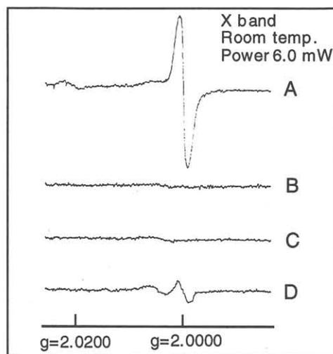
Fig. 5. ESR spectra of photo-CVD SiO<sub>2</sub> films. A: as-deposited, B: annealed in N<sub>2</sub>, C: annealed in O<sub>2</sub>, D: irradiated with UV light for 3 hours.
