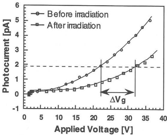
Fig. 1. Example of the voltage shift in photo I-V curves before and after irradiation with UV light.
