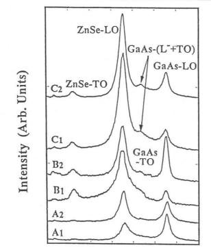
Fig.1. Raman spectra of ZnSe films grown on GaAs(100) substrates with S passivations. The samples signed A, B and C are for the GaAs substrates with semiinsulating, n-type doping concentration of  $1.0 \times 10^{16}$  and 1.3×10<sup>18</sup> cm<sup>-3</sup>, respectively. The samples signed 1 and 2 are passivated by (NH<sub>4</sub>)<sub>2</sub>S<sub>x</sub> and  $S_2Cl_2$ solutions, respectively.
