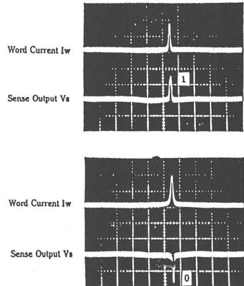
Figure 4. Pulse sequence of reading process.
