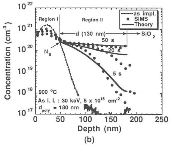
Fig. 1. Comparison between theoretical and experimental impurity profiles in polysilicon gate using a diffusion coefficient as a fitting parameter: (a) B; (b) As.
