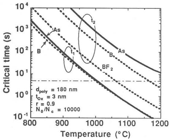
Fig. 4. Dependence of critical times on temperature.  $t_1$  is the critical time for impurity profile in polysilicon to be flat, and  $t_2$  is the critical time for impurity not to penetrate 3-nm-thick gate oxide.
