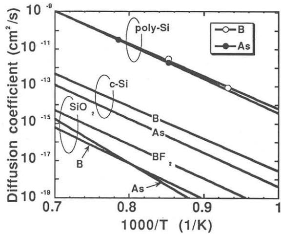
Fig. 3. Diffusion coefficient of B and As in polysilicon. Those in crystal Si and SiO<sub>2</sub> are also indicated.
