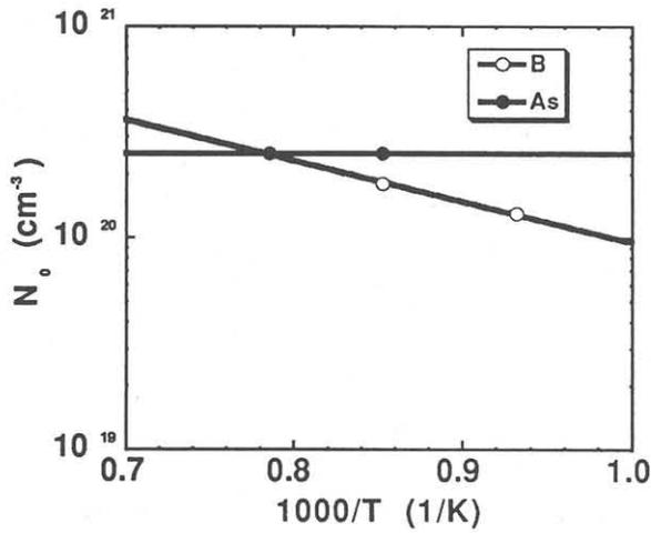
Fig. 2. Dependence of constant surface concentration  $N_0$  on temperature.
