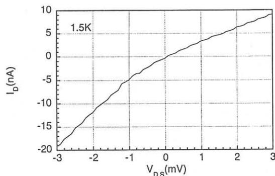
Fig. 5 Coulomb staircase at 1.5K.
