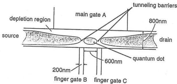
Fig. 2 SEM image and its schematic illustration of the fabricated IPG SET.
