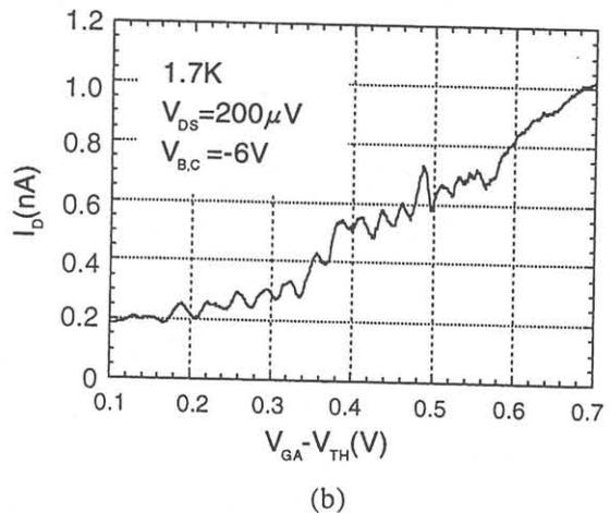
Fig. 4 Coulomb blockade oscillation at low temperature. The bias conditions are different in (a) and (b).
