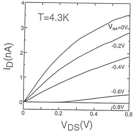
Fig 3 FET characteristic at 4.3K
