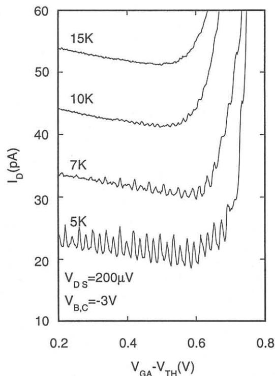
Fig. 6 Temperature dependence of Coulomb oscillation.
