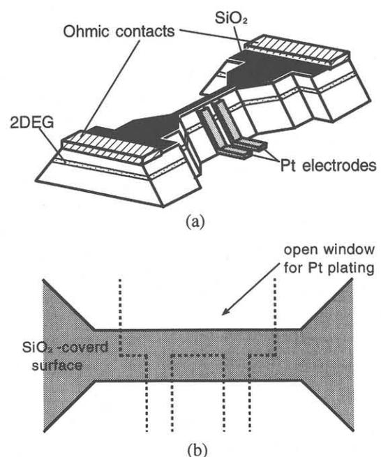
Fig. 1 (a) The scheme of single-electron transistor with Schottky IPGs. (b) Window pattern for Pt plating.
