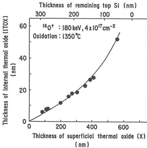
Fig. 2. Relationship between the thicknesses of internal thermal oxide and superficial thermal oxide formed by high-temperature oxidation at 1350°C. (After Nakashima et al.<sup>8)</sup>)
