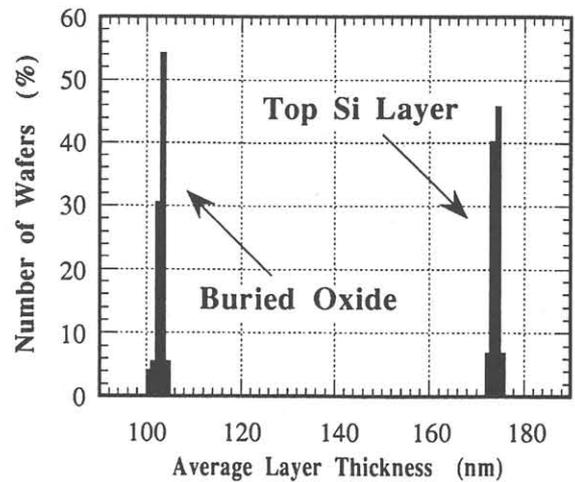
Fig. 4. "Wafer to wafer" uniformity of the top Si and BOX layers in the low-dose SIMOX wafers.
