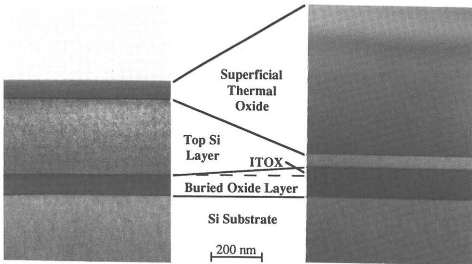
Fig. 1. XTEM micrographs of low-dose SIMOX wafers implanted with an oxygen dose of  $4 \cdot 10^{17}$  at/cm<sup>2</sup> at 180 keV. Left: before high-temperature oxidation. Right: after high-temperature oxidation. (After Nakashima et al.<sup>8)</sup>)
