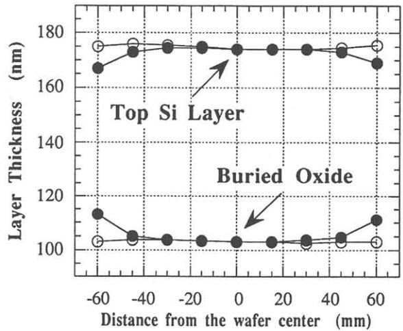
Fig. 3. Typical "on wafer" uniformity of the top Si and BOX layers in the low-dose SIMOX wafer, measured in two perpendicular directions.
