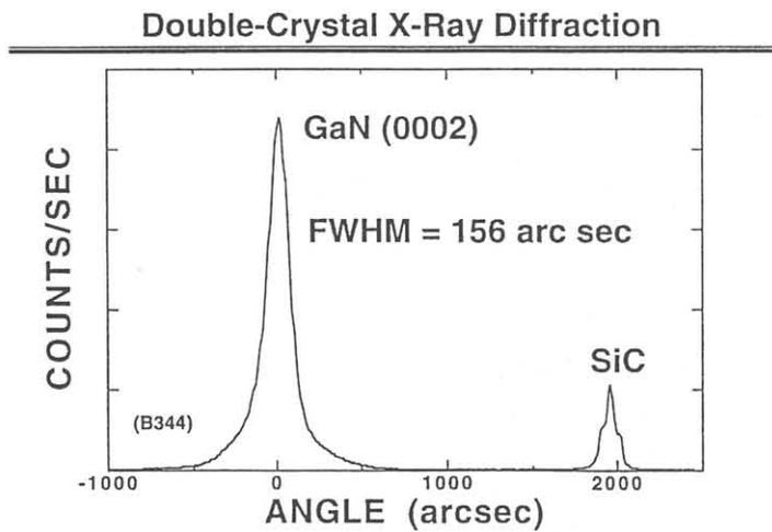
Figure 2. X-ray diffraction from MBE-grown GaN.
