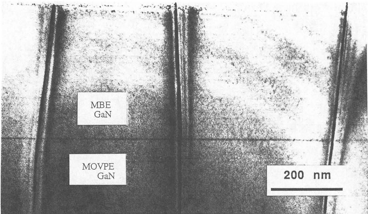
Figure 1. Vertical cross-section TEM of MBE-grown GaN on GaN/SiC substrate.
