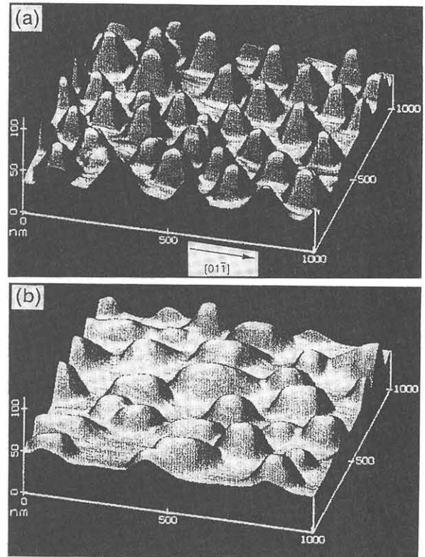
Fig. 4. AFM images of the structures formed on InP (311)B substrates.
