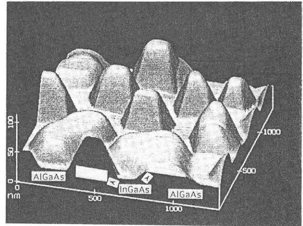
Fig. 3. AFM image of the initial stage.
