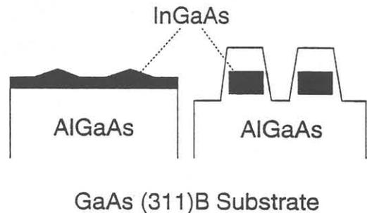
Fig. 1. Schematic growth mode.
