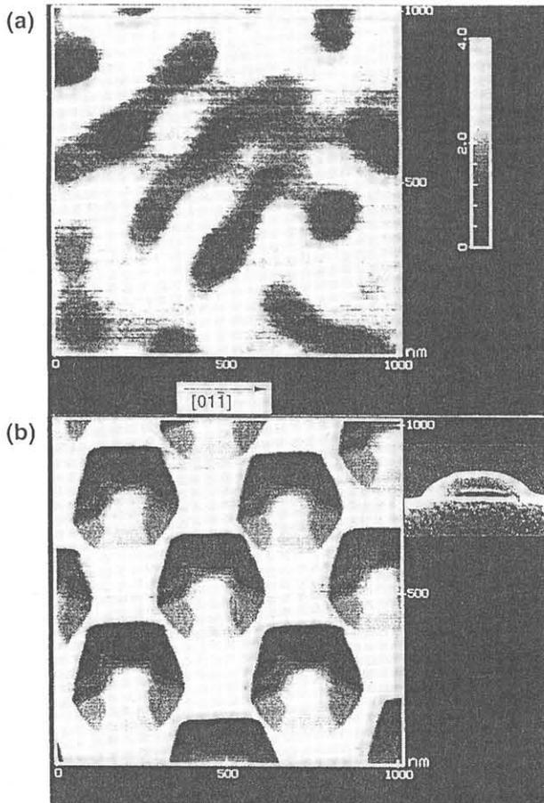
Fig. 2. AFM top views of (a) the modulated InGaAs layer and (b) the final AlGaAs microcrystals.
