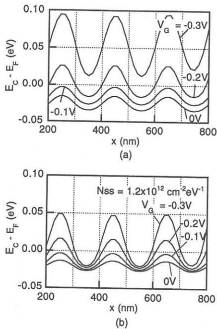
**Figure 2.** Calculated potentials at heterointerface of (a) the LSSL having controlled Schottky barriers and (b) conventional periodic split gate.
