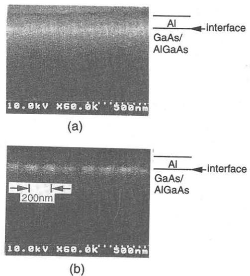
**Figure 4.** The cross sectional (a) SEM and (b) EBIC images.
