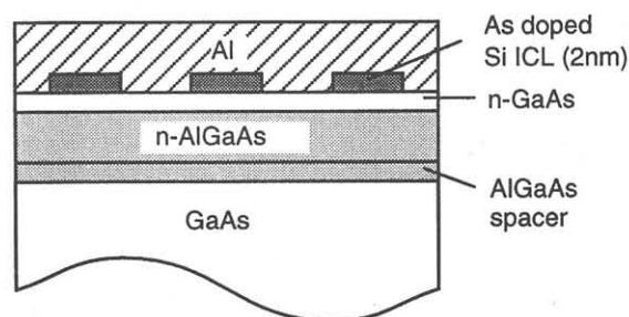
**Figure 1.** The new potential modulation structure for LSSL.
