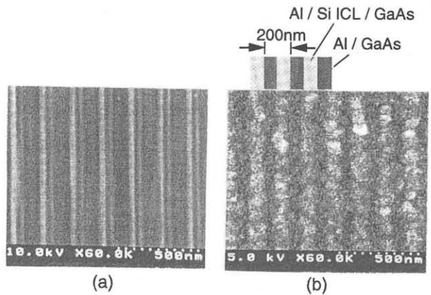
**Figure 3.** SEM images of (a) the basic pattern of the grating gate and (b) after metalization.
