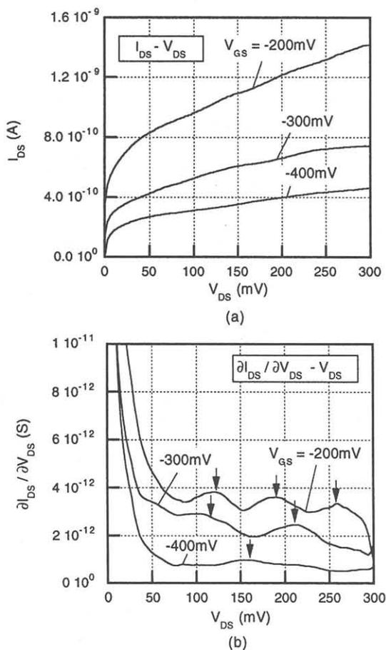
**Figure 6.** (a)  $I_{DS}-V_{DS}$  characteristics and (b) output conductance of the LSSL.
