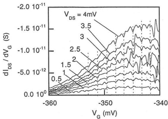
**Figure 5.** The transconductance characteristics of the LSSL.
