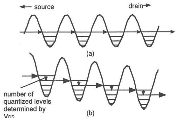
**Figure 7.** Sequential resonant tunneling model for the observed oscillatory behavior.
