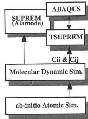
Fig. 4: Connection of tools in the hierarchical modeling of material coefficients  $C_{ii}$  and  $C_{ij}$ .
