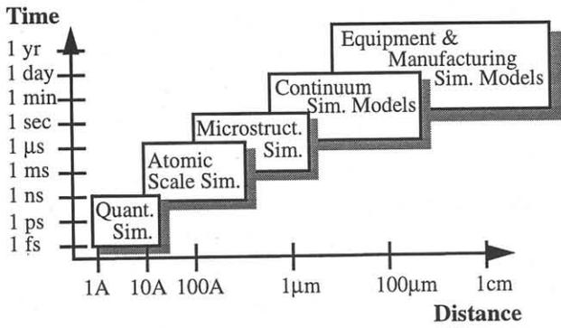
Fig1: Dimension and time scales in TCAD modeling.
