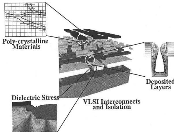
Fig. 5: A virtual-wafer model of cell-level interconnects for an SRAM cell.
