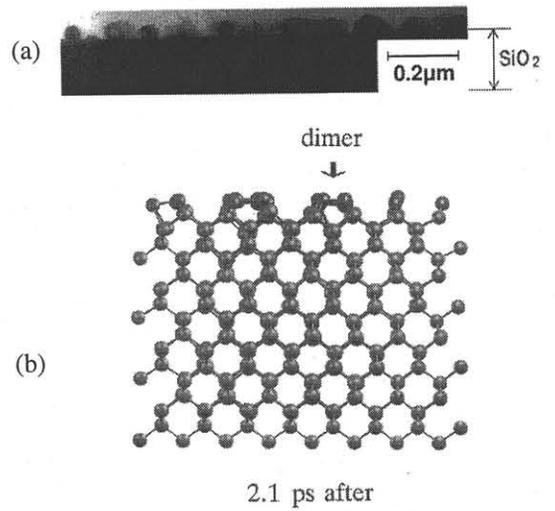
Fig. 3: Nucleation of silicon islands from deposited amorphous silicon substrate: (a) TEM image; (b) molecular dynamic simulation.
