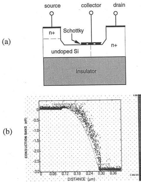
Fig. 2: A novel hot electron structure in silicon (HESS) device: (a) the schematic cross-section; (b) Monte Carlo results of carrier distributions at the collector surface.
