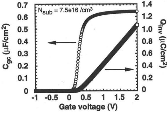
Fig. 3. Dependence of  $C_{gc}$  and  $Q_{inv}$  on gate voltage.
