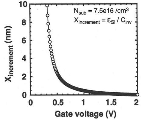
Fig. 4. Dependence of  $X_{increment}$  on gate voltage.
