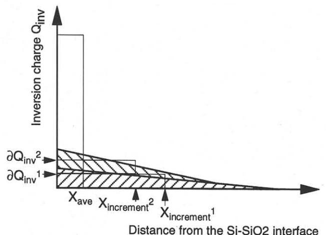
Fig. 2. Schematic representation of extraction method.
