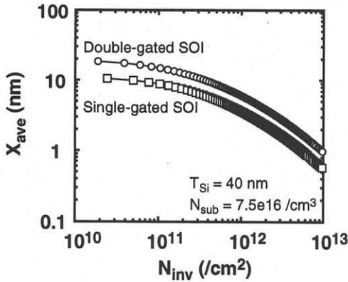
Fig. 7. Comparison of inversion layer thickness.
