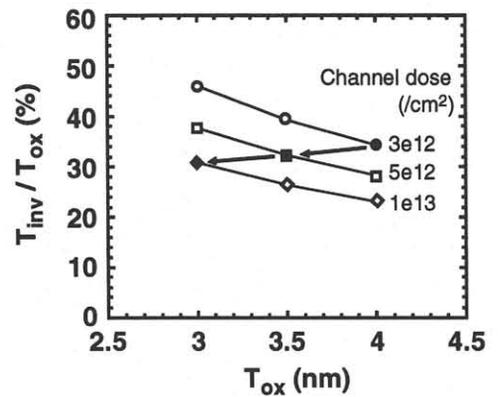
Fig. 6. Ratio of inversion layer thickness to gate oxide thickness.
