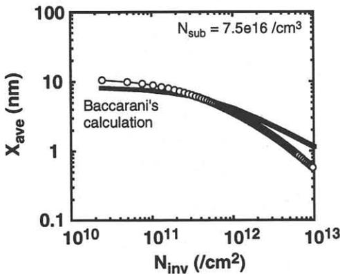
Fig. 5. Dependence of inversion layer thickness on inversion charge density.
