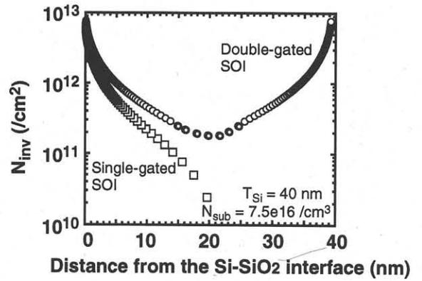
Fig. 8. Inversion charge profile in the Si layer.
