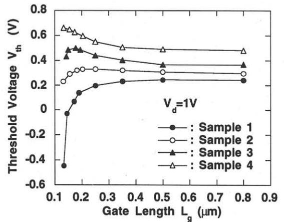
**Fig. 4.** Experimental threshold voltage  $V_{th}$  at  $V_d=1 \text{ V}$  versus gate length  $L_g$  for samples with different doses of boron at 10 keV.
