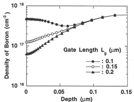
**Fig. 2.** Depth profile of boron under center of gate simulated by SUPREM-4 for each gate length. Tilted II of boron ( $\theta=45^\circ$ ) at 10 keV with a dose of  $4 \times 10^{12} \text{ cm}^{-2}$  is assumed.
