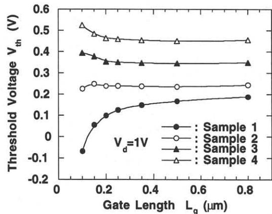
**Fig. 5.** Simulated threshold voltage  $V_{th}$  at  $V_d=1 \text{ V}$  versus gate length  $L_g$ . The result of process simulation by SUPREM-4 (see Fig. 2) was used in the 2-D device simulation. Assumed conditions for tilted II and other processes were same as the fabricated samples.
