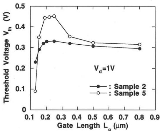
Fig. 6. Experimental threshold voltage  $V_{th}$  at  $V_d=1\text{ V}$  versus gate length  $L_g$  for samples with different II energies.
