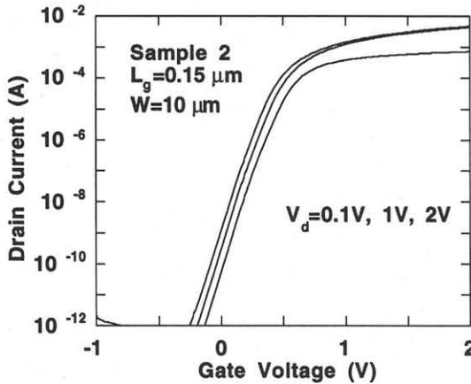
**Fig. 3.** Subthreshold I-V characteristics of Sample 2 at  $V_d=0.1 \text{ V}$ ,  $1 \text{ V}$ , and  $2 \text{ V}$ . Gate length  $L_g$  is  $0.15 \mu\text{m}$ .
