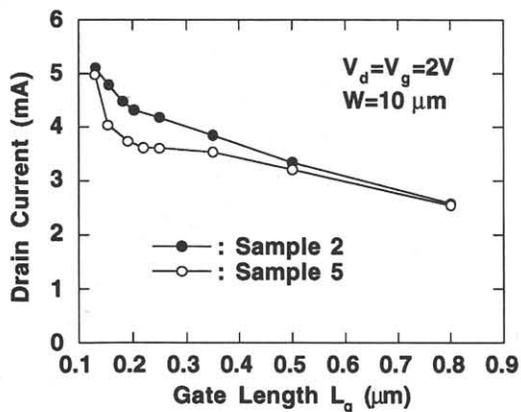
Fig. 7. Experimental drain current  $I_d$  at  $V_d=V_g=2\text{ V}$  in Samples 2 and 5.
