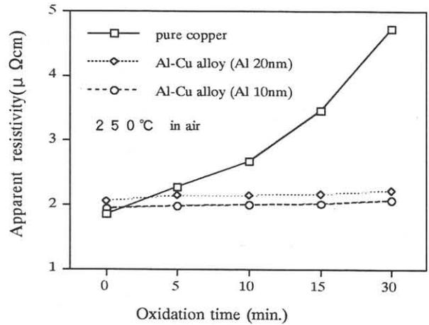
Fig. 6 Oxidation time vs. Apparent resistivity
