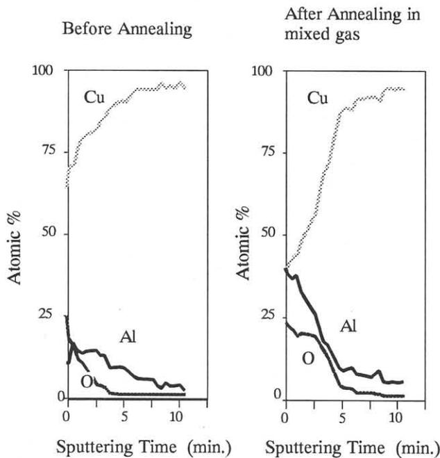
Figs. 5 AES depth profile before and after annealing in mixed gas
