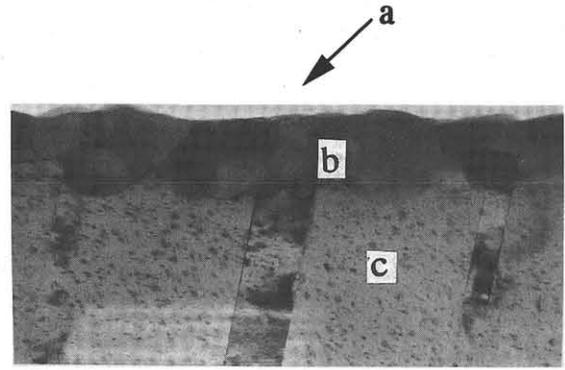
Fig.3 Cross-sectional TEM image of the surface passivated copper film
