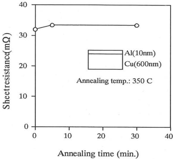
Fig.2 Sheet resistance vs. annealing time
