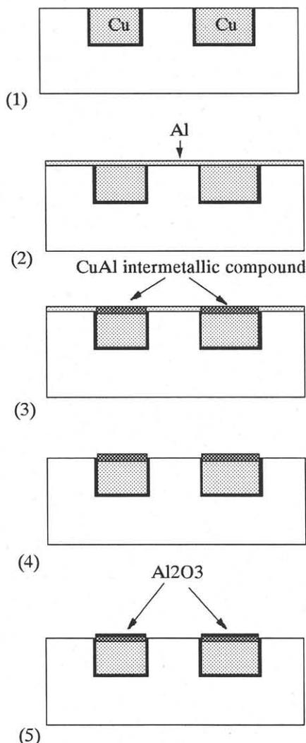
Fig. 1 Process sequence of self aligned passivation
