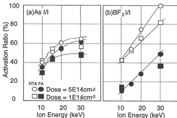
Fig. 1 Dependence of carrier activation ratio on the ion energy. (a) As ion implantation, (b) BF<sub>2</sub> ion implantation
