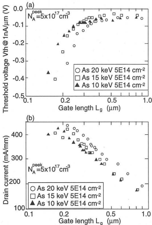
Fig. 4 Gate length ( $L_g$ ) dependence of n-MOSFET characteristics
