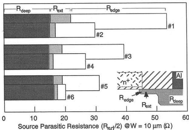
Fig. 5 Source parasitic resistance ( $R_{sd}/2$ ) as a function of ion energy. RTA was carried out at 950°C for 10 s.
