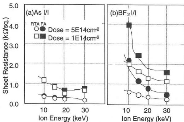
Fig. 2 Dependence of sheet resistance on the ion energy. (a) As ion implantation, (b) BF<sub>2</sub> ion implantation
