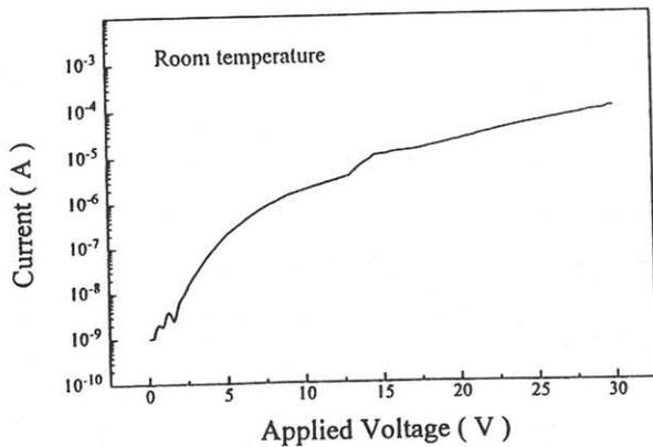
Fig. 2(b) The current density vs. applied voltage characteristics of the proposed PS-based LED without a-Si:H layer.
