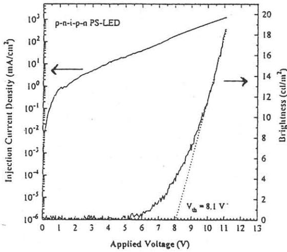
Fig. 2(a) The current density and brightness vs. applied voltage for the proposed PS-based LED.
