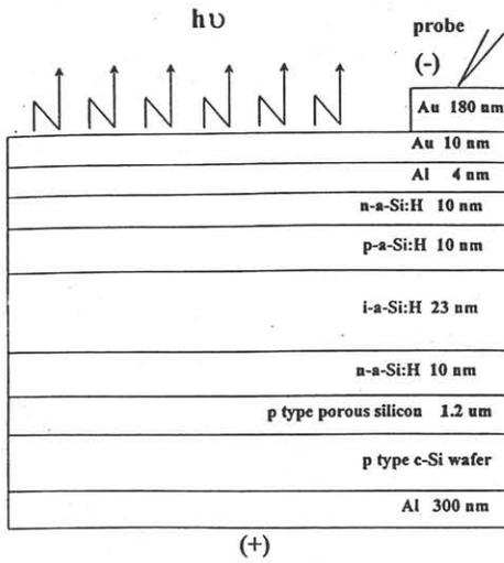
Fig. 1 The schematic cross-section of the proposed PSLED
