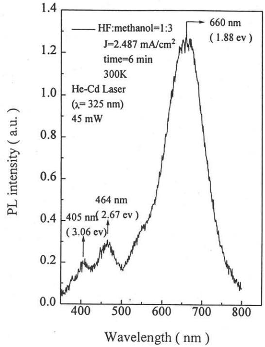
Fig. 3 The PL spectrum of the as-anodized PS.
