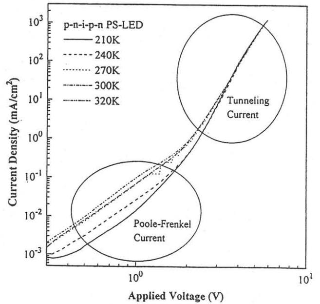
Fig. 4 The plot  $\log(J)$  vs.  $\log(V)$  for the proposed PS-based LED under different temperatures.
