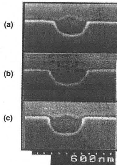
Fig. 2. Field oxide profile after gate cleaning. Overetching in isolation etching : (a), (b) : 50 %, (c) : 100 %, overetching in spacer etching : (a), (c) : 170 %, (b) : 230 %
