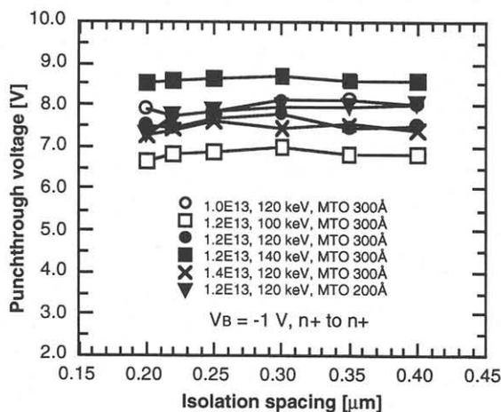
Fig. 5. Punchthrough voltage vs. isolation spacing with various channel stop boron implantation conditions and MTO thicknesses.
