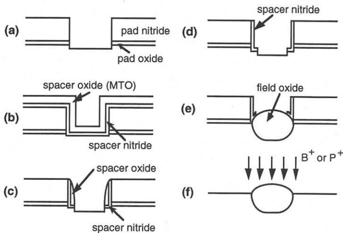
Fig. 1. A process sequence of the DS-LOCOS : (a) formation of conventional LOCOS structure with overetching in isolation etching; (b) deposition of spacer nitride and spacer oxide; (c) spacer formation with overetching; (d) spacer oxide removal; (e) field oxidation; and (f) channel stop implantation through field oxide.
