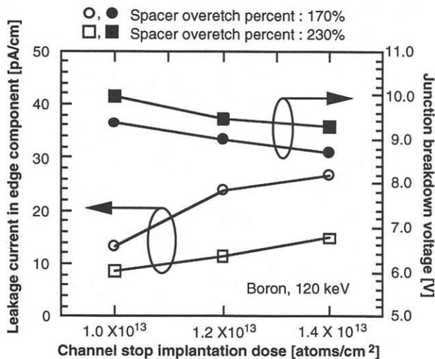
Fig. 4. Junction leakage current and breakdown voltage as a function of channel stop implantation dose with variation of spacer overetch percent.
