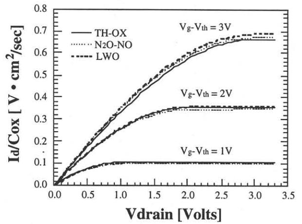
(b) Long Channel nMOSFET (W/L = 50  $\mu\text{m}/10 \mu\text{m}$ )
