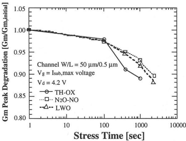
Fig.6. Gm peak degradation of nMOSFET under avalanche hot electron stress
