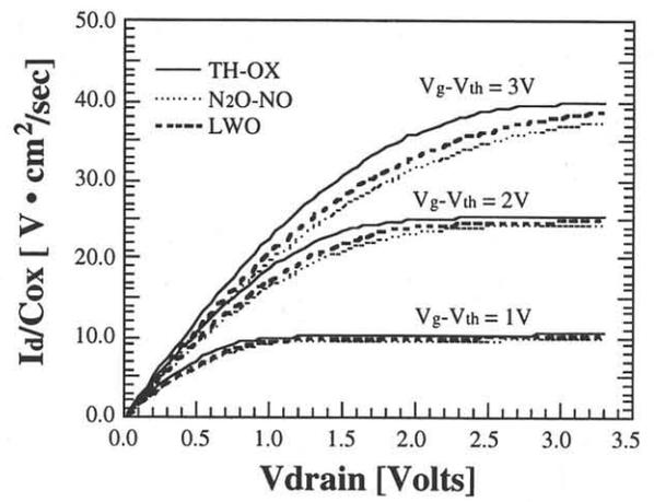
(a) Short Channel nMOSFET (W/L = 50  $\mu\text{m}/0.6 \mu\text{m}$ )
