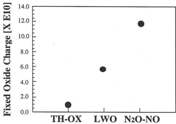
Fig.3. Fixed oxide charges of various oxidation conditions
