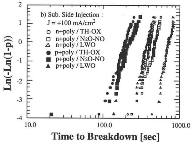
Fig.2. TDDB characteristics for 70 Å thermal oxide and nitrided oxides under gate side (a) and substrate side injection (b) (n+poly : POCl<sub>3</sub> doped poly p+poly : BF<sub>2</sub> implanted poly)
