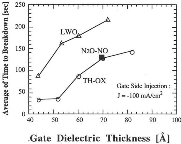
Fig.1. TDDB characteristics of thin thermal oxides and nitrided oxides under gate side injection
