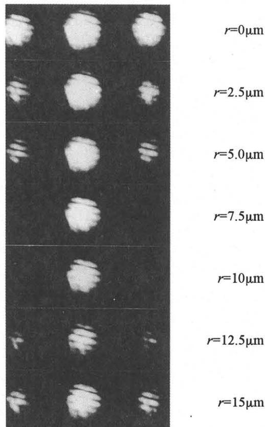
**Fig. 4** Laser beam diffraction patterns as a function of the relative position  $r$ . The zero point  $r=0$  was determined such that the intensities of  $\pm 1\text{st}$  order spots became maximum.
