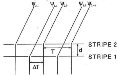
Fig. 6 The model for theoretical calculation on the intensities of diffraction spots. It is assumed that the beams diffracted by stripe1 ( $\psi_{1,n}$ ) and stripe2 ( $\psi_{2,n}$ ) are interfered.
