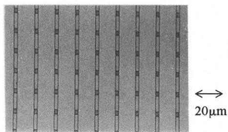
**Fig. 3** The top view micrograph of a pair of stacked stripes which corresponds to Fig. 1(iv). It is seen that the uniform stacking has been successfully achieved.
