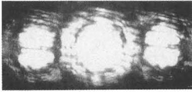
Fig. 5 The photograph of  $\pm 1$ st and 0th order diffraction spots for  $\theta=0.6^\circ$ . The dark line is observed in the  $\pm 1$ st order spots.
