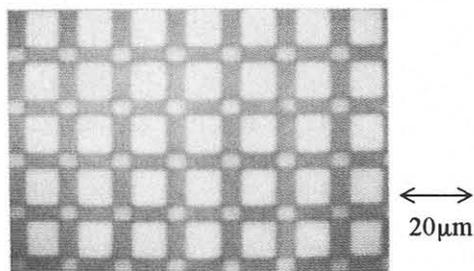
**Fig. 2** Transmission infrared micrograph of the wafer-bonded striped structures. The bright and dark areas correspond to the bonded and the etched areas, respectively.
