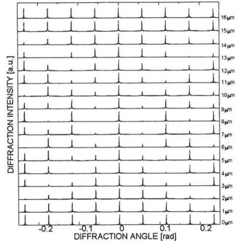
Fig. 7 Calculated results of  $-4$ th to  $4$ th order diffraction spots as a function of  $\Delta T$ .
