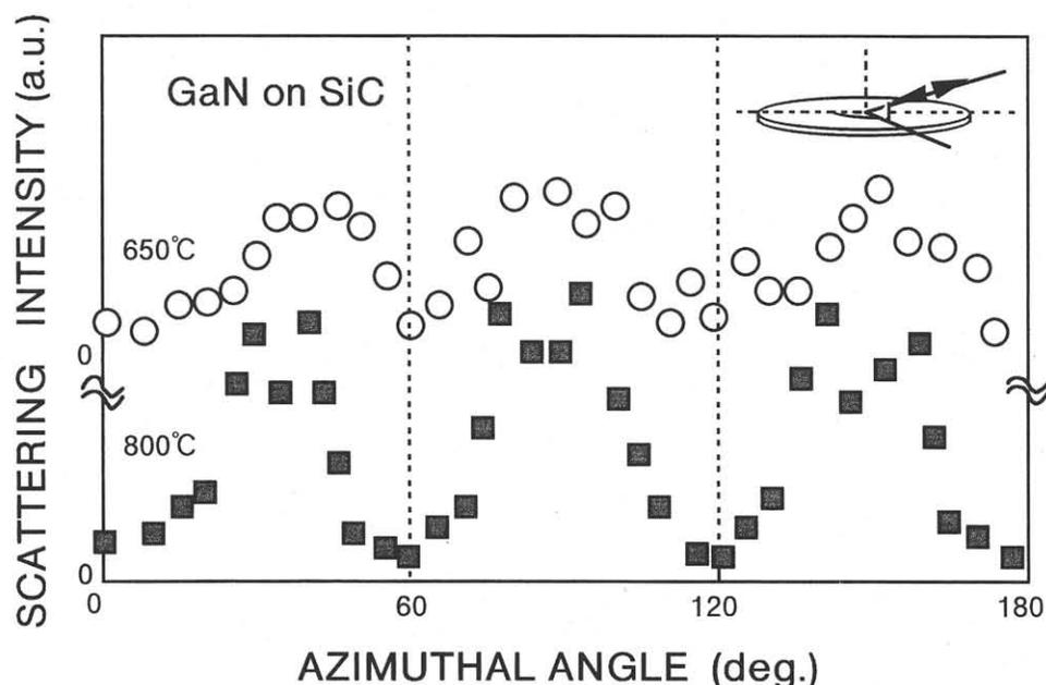
Figure 4. The azimuthal-angle scans of scattering intensity from Ga atoms.
