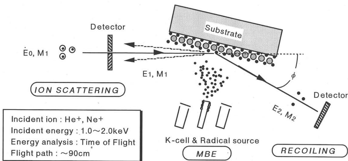
Figure 1. Schematics of MBE-ISARS apparatus.
