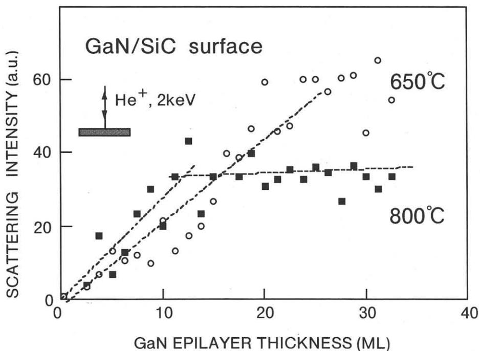
Figure 3. The [0001]-aligned scattering intensity from Ga atoms as a function of GaN epilayer thickness.
