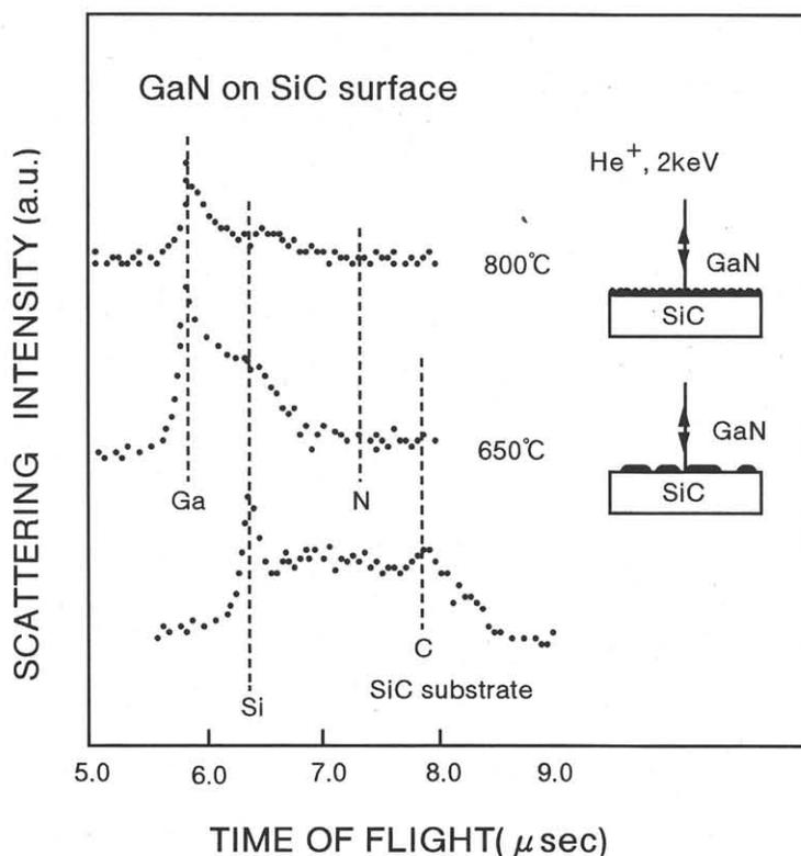
Figure 2. TOF spectra of GaN on SiC MBE grown surface at several growth temperature.
