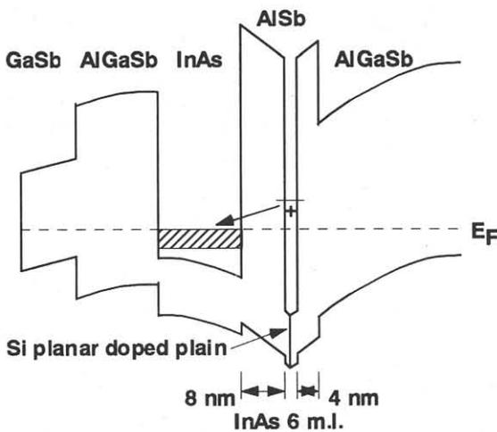
Fig. 2 Energy band diagram of the InAs/AlGaSb structure with a Si planar doped ultrathin InAs electron supplying layer. Most of electrons transfer from the elevated donor states in the ultrathin InAs quantum well into the thick InAs channel layer.
