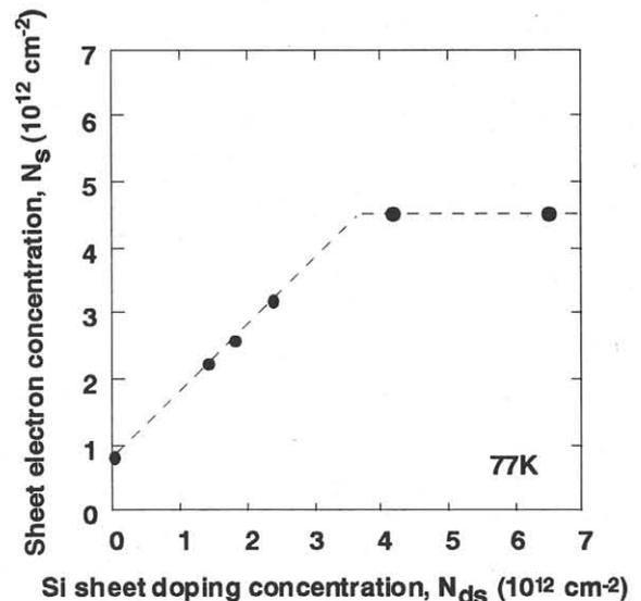
Fig. 3 Two-dimensional electron gas concentration,  $N_s$ , as a function of Si sheet doping concentration,  $N_{ds}$ , measured by van-der Pauw method at 77K.
