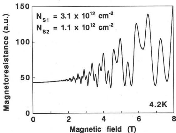
Fig. 4 Shubnikov-de Haas oscillations for  $N_{ds} = 4.1 \times 10^{12} \text{ cm}^{-2}$ . Two oscillation components correspond to the 2DEG concentrations of  $3.1 \times 10^{12} \text{ cm}^{-2}$  and  $1.1 \times 10^{12} \text{ cm}^{-2}$ .
