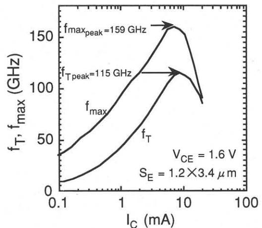
Fig. 6. Dependence of  $f_T$  and  $f_{max}$  on the collector current of a fabricated HBT with a base doping level of  $1 \times 10^{20} \text{ cm}^{-3}$ .
