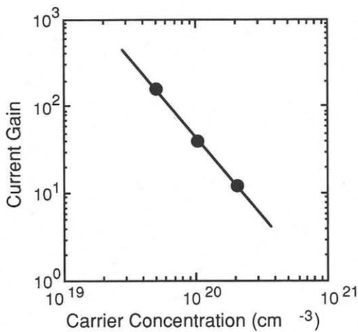
Fig. 5. Current gain as a function of carrier concentration at a collector current of 10 mA.
