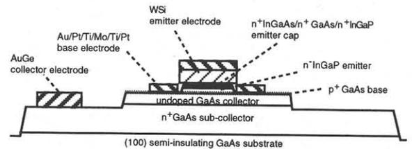
Fig. 3. Schematic cross section of the fabricated HBT.
