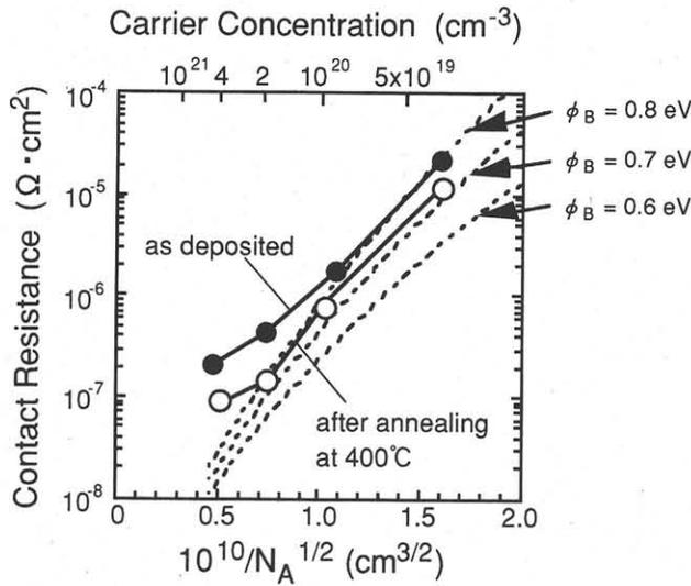
Fig. 2. Contact resistance as a function of carrier concentration  $N_A$  in 30-nm-thick GaAs.
