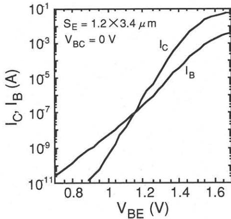
Fig. 4. Gummel plot of the fabricated HBT with a base doping level of  $1 \times 10^{20} \text{ cm}^{-3}$ .
