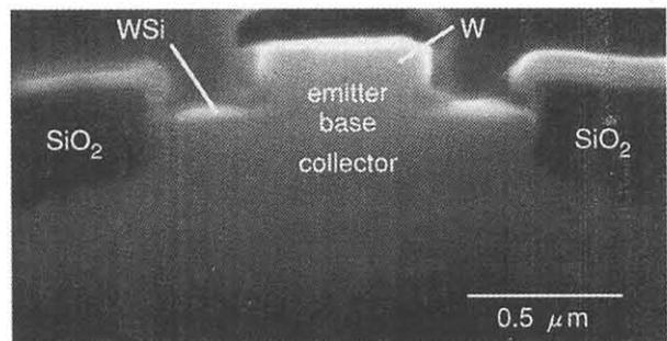
Fig. 1. SEM cross section of a WSi base electrode structure.
