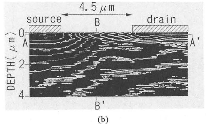
FIG.5 (a) Measured two-dimensional image of the electrostatic potential. The bias voltage is 1.5 V. (b) Corresponding contour lines. The voltage step of each contour line is 40 mV.
