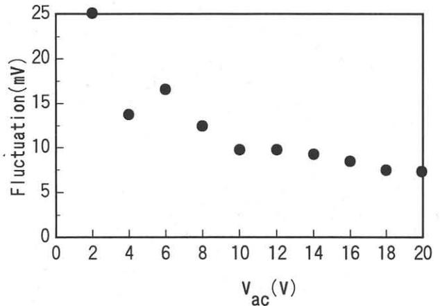
FIG.4 Dependence of voltage fluctuation on the alternating voltage amplitude.
