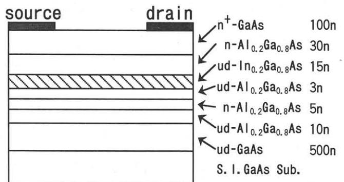
FIG.2 Schematic cross section of the measured device.
