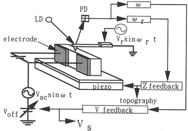
FIG.1 Schematic diagram of the KFM measurement system.
