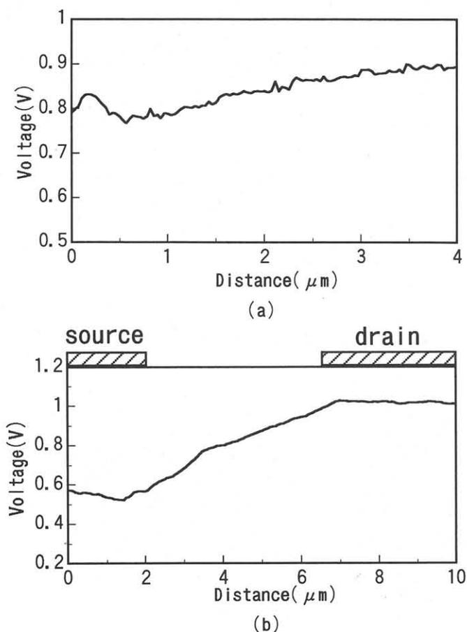
FIG.6 Potential distribution along the BB' line (a) and the AA' line (b) of Fig.5(b).
