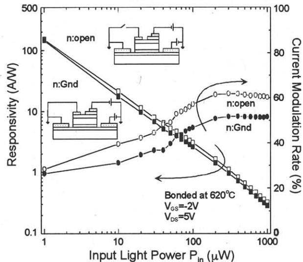
Fig.4. Input light power dependence of the responsivity and the current modulation rate for the sample directly bonded at 620°C.
