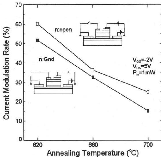
Fig.3. Relationship between current modulation rate of optically controlled FET and bonding temperature when input light power was 1mW.
