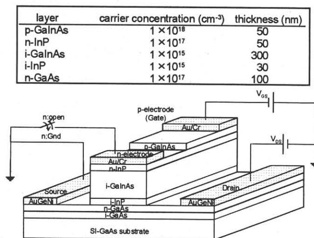
Fig.1. Schematic structure of optically controlled FET in which i-InP bonding layer of absorption region and n-GaAs layer of FET region were directly bonded.
