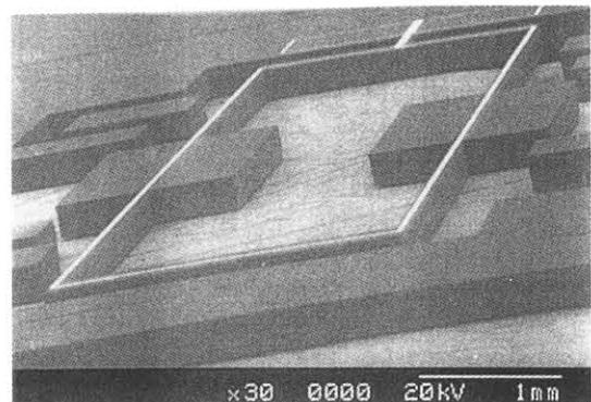
Fig.3 Silicon resonant angular rate sensor and silicon tuning fork formed by deep RIE
