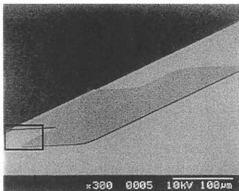
Fig.1 Thin silicon cantilever attached on a metallized glass plate with narrow gap
