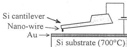
Fig.2 Silicon nanowire grown at the tip of a cantilever
