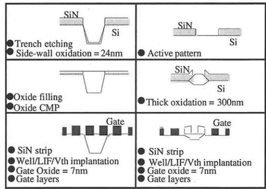
Fig.5 A simplified STI process schematics used in this work
