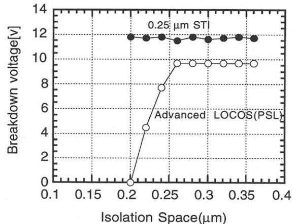
Fig.1 Isolation breakdown voltage vs. STI & LOCOS.
