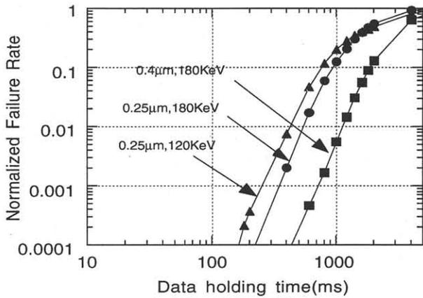
Fig.7 Data retention times vs different trench depth and doping structures of STI in stack DRAM
