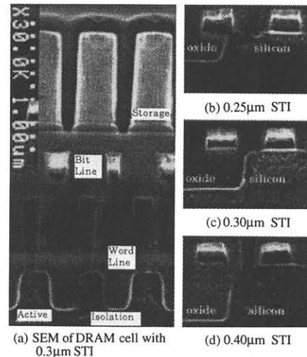
Fig.6 Cross sectional SEM images of cell structure and STI profiles having 0.25/0.3/0.4 $\mu$ m trench depth
