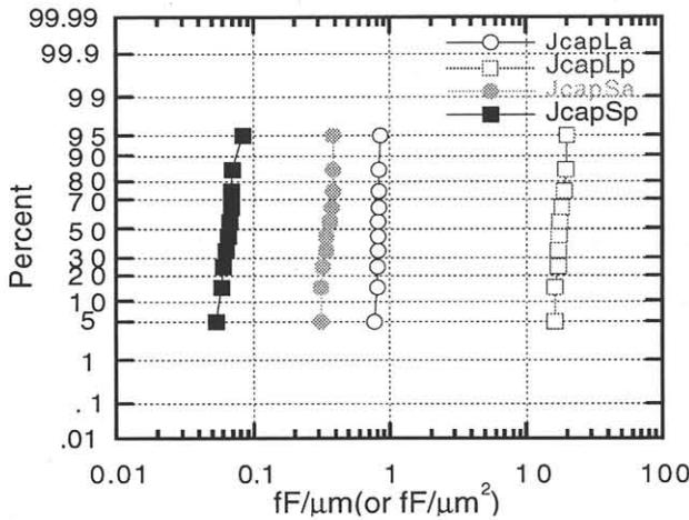
Fig.3 Junction capacitances vs. STI and LOCOS
