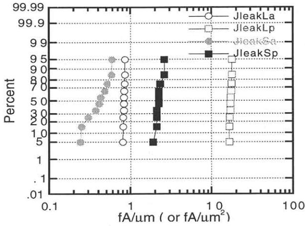
Fig.2 Junction leakage currents vs. STI and LOCOS
