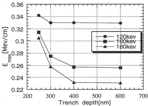
Fig.8 Maximum junction electric field of cell storage node as various trench depth and doping structures.
