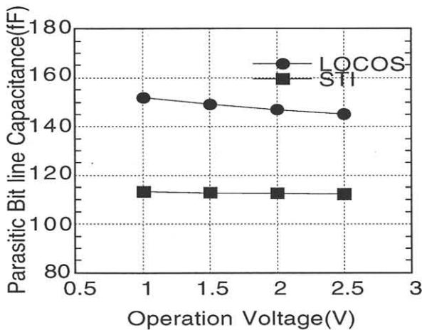
Fig.4 Bit line capacitances(Cb) vs. STI and LOCOS as function of operation voltage(256bits/bit line)
