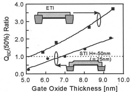
Figure 9. Gate oxide thickness dependence of  $Q_{BD}$  in cumulative failure 50 % normalized for  $Q_{BD}$  at  $t_{ox} = 7 \text{ nm}$  in STI. DC 0.3 A/cm<sup>2</sup> was injected into the gate. The capacitor area is 0.10 mm<sup>2</sup> and the perimeter is 0.13 mm.
