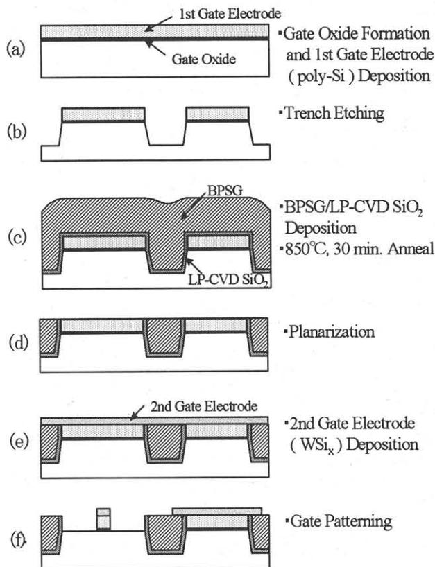
Figure 1. Elevated Trench Isolation (ETI) process flow.
