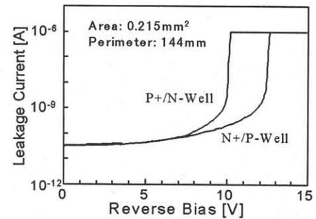
Figure 5. Junction leakage current characteristics for ETI
