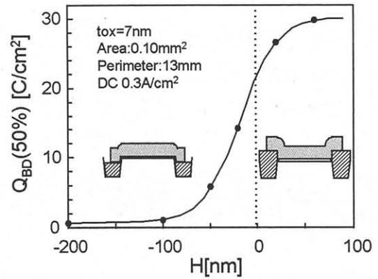
Figure 8.  $\text{SiO}_2$  height ( $H$ ) from active area dependence of  $Q_{BD}$  in cumulative failure 50 %.
