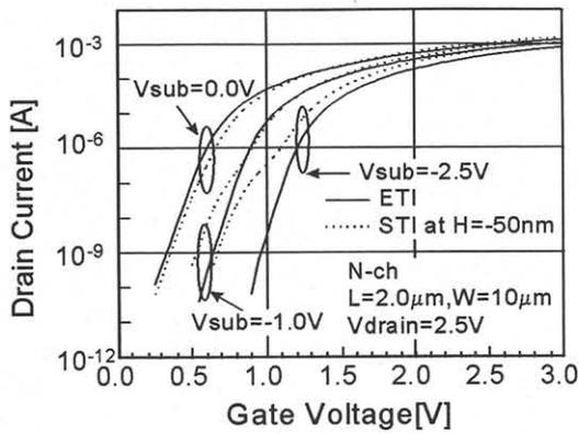
Figure 6. Subthreshold behavior on n-MOSFET.
