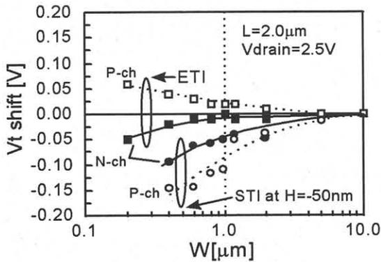
Figure 7. Channel width ( $W$ ) dependence of  $V_t$  shift ( $|V_t| - |V_t[W=10 \mu\text{m}]|$ ) for n-MOSFET.
