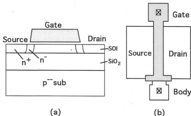
Fig.1 Cross-sectional and plane view of SOI MOSFET with body terminal.
