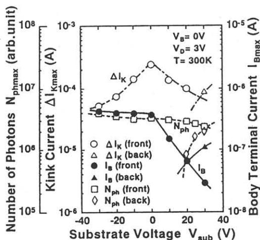
Fig.7 Substrate voltage dependence of maximum body terminal current, kink current and photon number.
