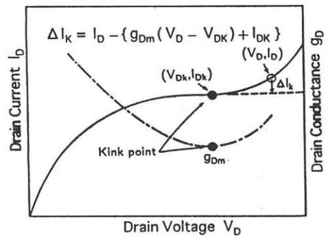
Fig.2 Drain conductance method.
