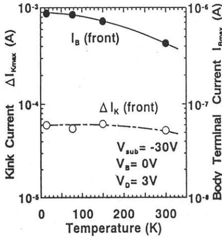
Fig.8 Temperature dependence of body terminal current and kink current at  $V_{sub}=-30V$ .
