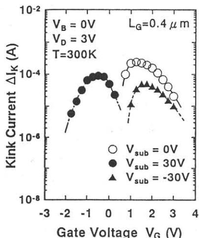
Fig.4 Gate voltage dependence of kink current.
