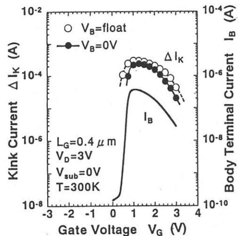
Fig.3 Gate voltage dependences of kink current and body terminal current.
