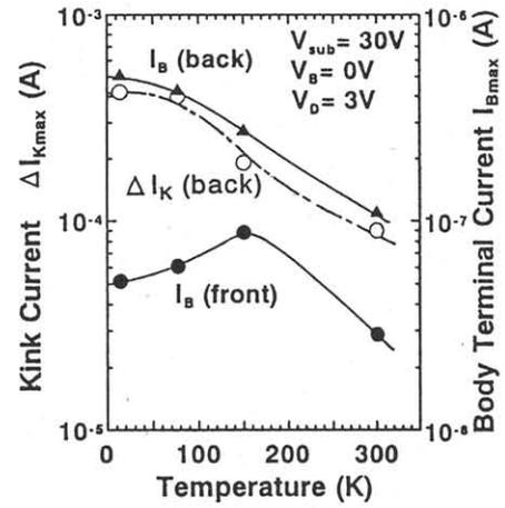
Fig.10 Temperature dependence of body terminal current and kink current at  $V_{sub}=+30V$ .
