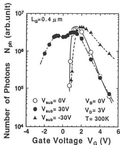
Fig.6 Gate voltage dependence of emitted photon number.
