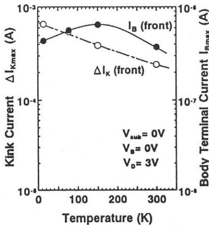
Fig.9 Temperature dependence of body terminal current and kink current at  $V_{sub}=0V$ .
