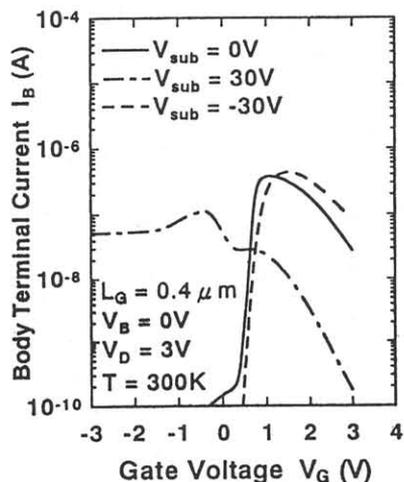
Fig.5 Gate voltage dependence of body terminal current.
