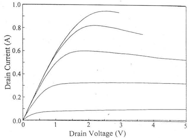
Fig. 4. Current-voltage (I-V) characteristics of atomic-planar-doped AlGaAs/InGaAs quantum-well HEMT. Top curve is  $V_{gs} = +1.0V$ ,  $V_{gs}$  step =  $-0.5V$ .
