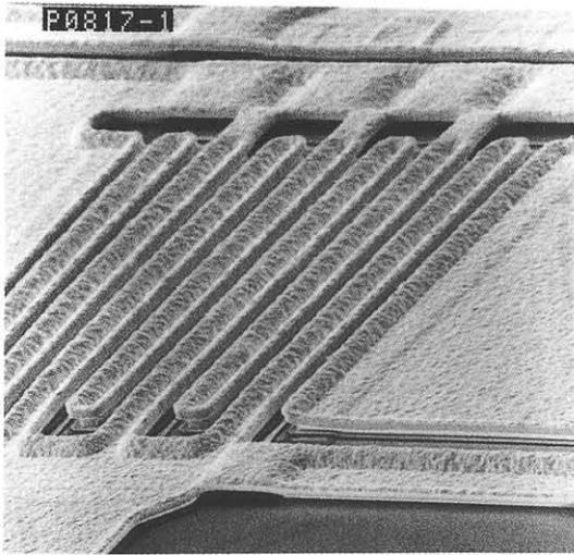
Fig. 2. Air bridges of source/drain fingers.
