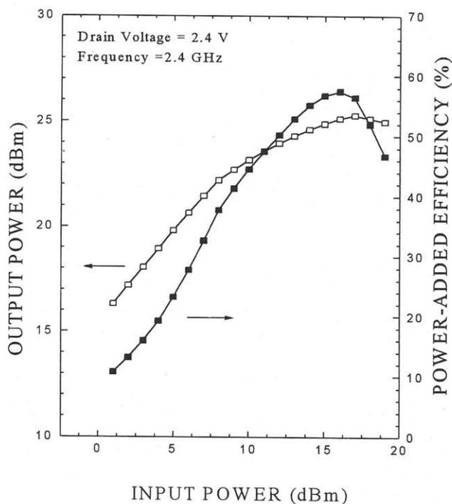
Fig. 6 Output power and power-added-efficiency as a function of input power at a drain bias of 2.4V. The measurement frequency is 2.4 GHz.
