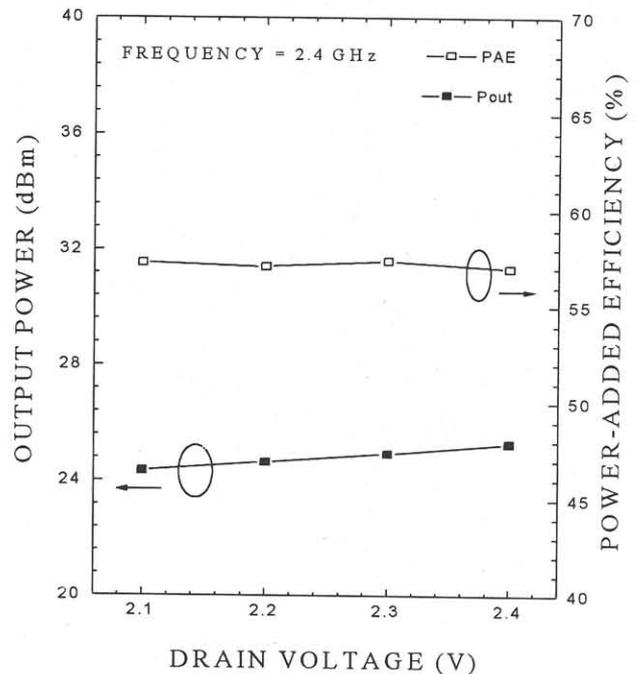
Fig. 7. Output power ( $P_{out}$ ) and power-added-efficiency (PAE) as a function of drain voltage. The measurement frequency is 2.4 GHz.
