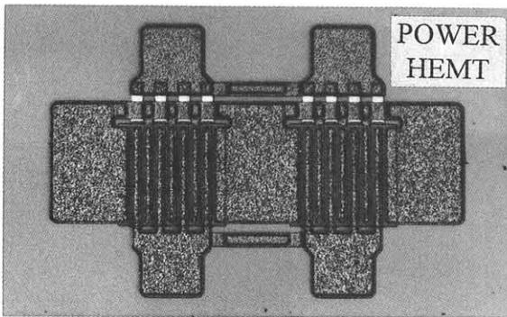
Fig. 3. Atomic-planar-doped AlGaAs/InGaAs quantum-well HEMT with 2mm gate width.
