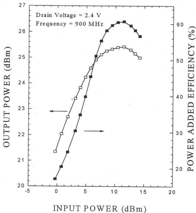
Fig. 5 Output power and power-added-efficiency as a function of input power at a drain bias of 2.4V. The measurement frequency is 900 MHz.
