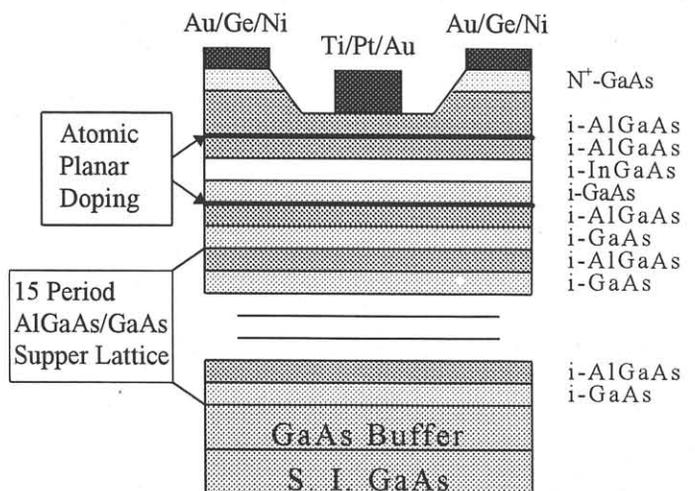
Fig. 1. Atomic-planar-doped AlGaAs/InGaAs quantum-well HEMT structure.
