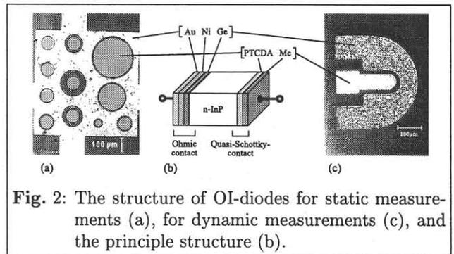
Fig. 2: The structure of OI-diodes for static measurements (a), for dynamic measurements (c), and the principle structure (b).
