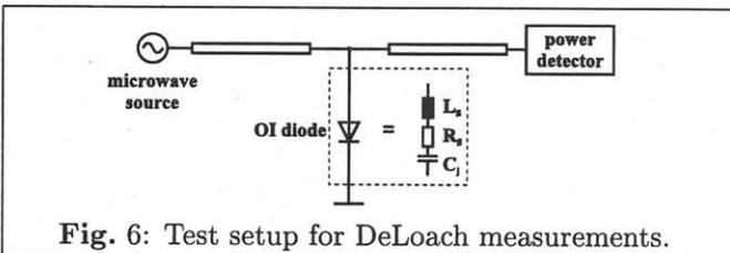
Fig. 6: Test setup for DeLoach measurements.
