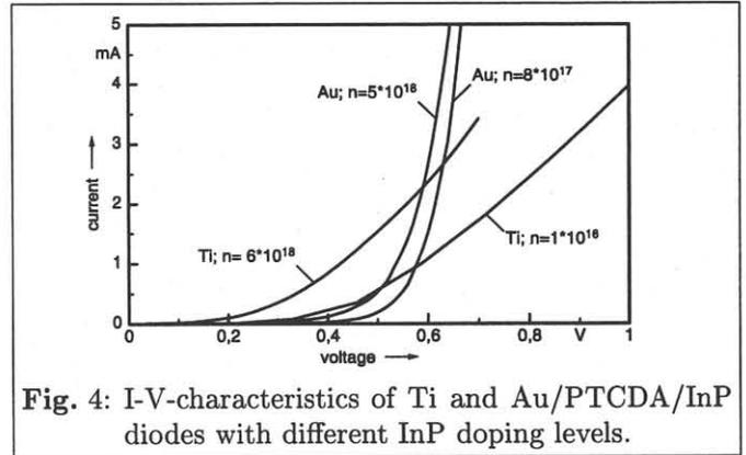
Fig. 4: I-V-characteristics of Ti and Au/PTCDA/InP diodes with different InP doping levels.
