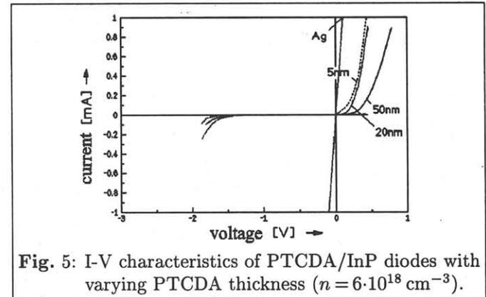
Fig. 5: I-V characteristics of PTCDA/InP diodes with varying PTCDA thickness ( $n = 6 \cdot 10^{18} \text{ cm}^{-3}$ ).
