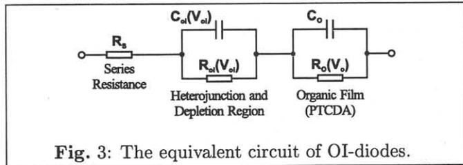
Fig. 3: The equivalent circuit of OI-diodes.
