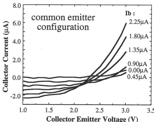
Fig.4 Output characteristics of the device of common emitter configuration.
