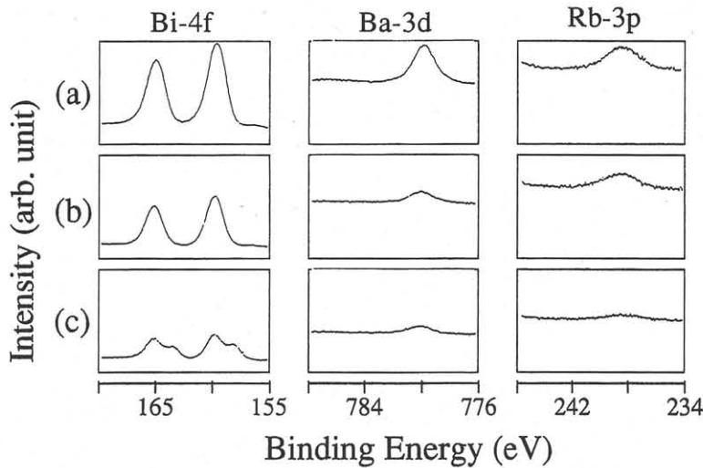
Fig.2 Bi-4f, Ba-3d and Rb-3p XPS spectra from BRBO thin films.
