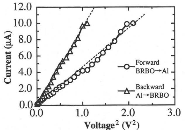
Fig.3 Diode characteristics of the Al/ $\text{Al}_2\text{O}_3$ /BRBO junction.
