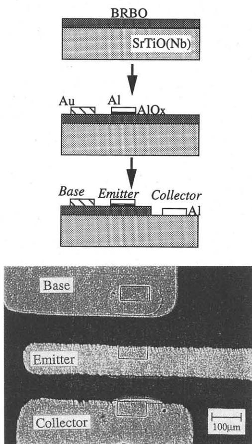
Fig.1 A schematic fabrication process and a top view of the Al/Al<sub>2</sub>O<sub>3</sub>/(Ba,Rb)BiO<sub>3</sub>/SrTiO<sub>3</sub>(Nb) device.
