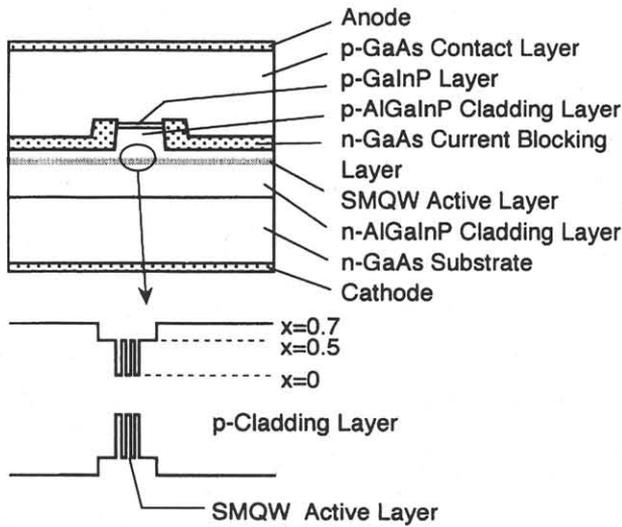
Fig. 2. Schematic cross section and band diagram of the laser.
