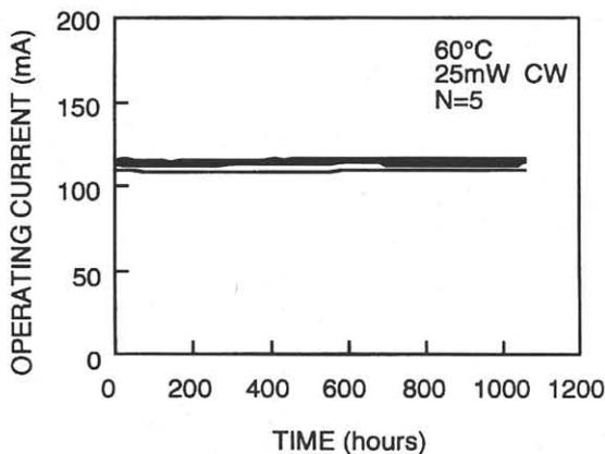
Fig. 5. Life test results at 60°C under a constant output power of 25mW.
