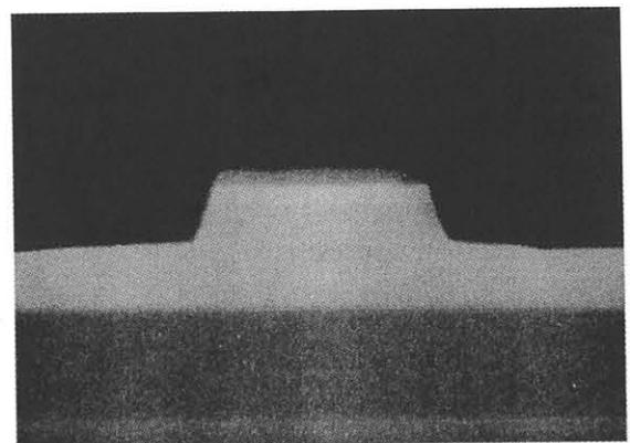
Fig. 1. Scanning electron microscope photograph of etched laser mesa.
