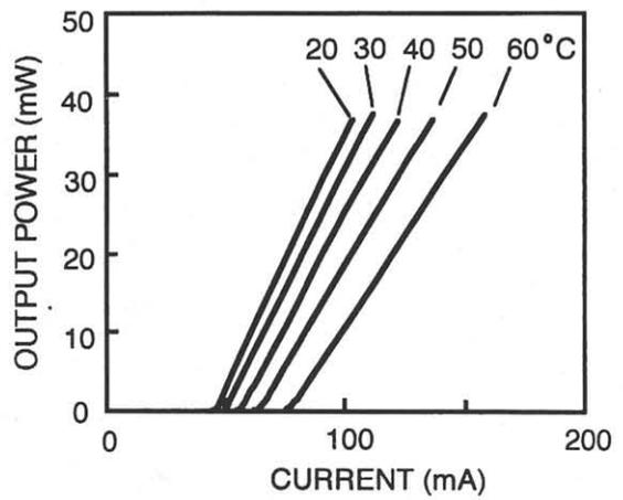
Fig. 3. Temperature dependence of output power vs current characteristics of 6%/80% coated laser.
