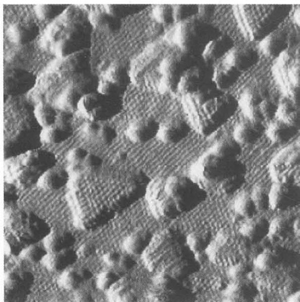
Fig.1 UHV-STM observation of H-terminated Si(111) surface by dry treatment. 20x20nm
