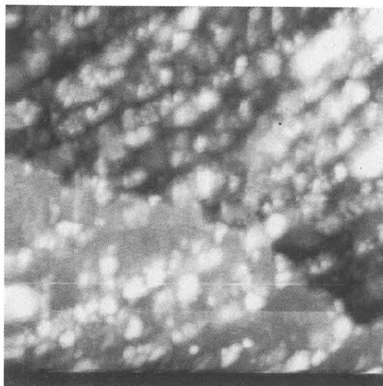
Fig.2 UHV-STM observation of Ni-deposited Si(111) substrate annealed at 400°C which was H-terminated by dry treatment. 50x50nm
