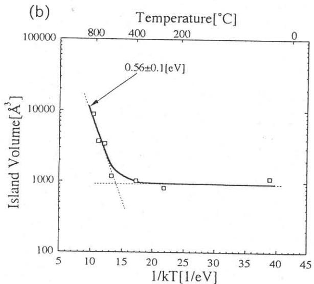
Fig.6 Islands volume as a function of reciprocal of temperature. (a) on Si (111)-7x7, (b) on H-terminated Si(111)-1x1.
