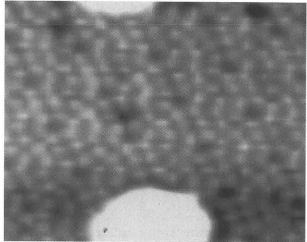
Fig.5. UHV-STM observation of Ti-deposited Si(111) surface annealed at 760°C. 10x8nm
