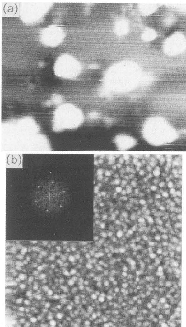
Fig.4 UHV-STM observation of Ti-deposited Si(111) surface at a room temperature.
