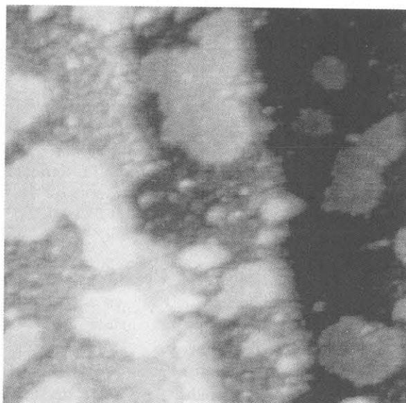
Fig.3 UHV-STM observation of Ni-deposited Si(111) substrate annealed at 400°C which had 7x7 structure before deposition. 50x50nm
