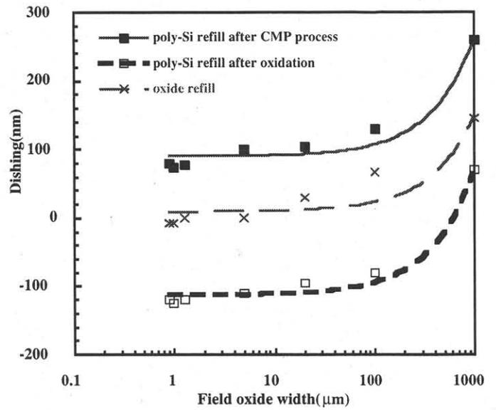
Fig. 4 The dishing results of shallow trenches.
