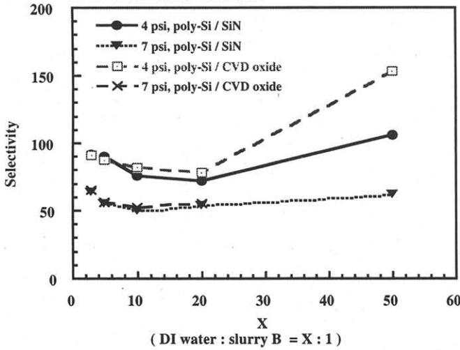
Fig. 2(b) The etch selectivity of poly-Si to CVD oxide and SiN.
