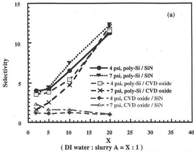
Fig. 2(a) The etch selectivity of CVD oxide to SiN, and poly-Si to CVD oxide and SiN.
