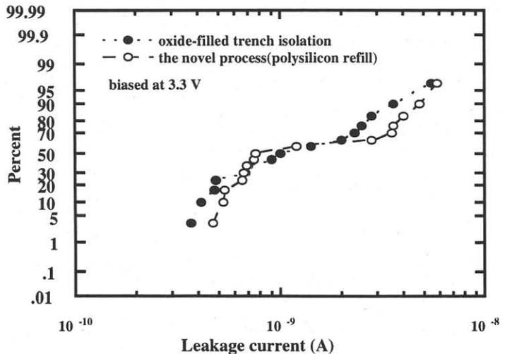
Fig. 6 The leakage current distribution of the n<sup>+</sup>/p junction diodes.
