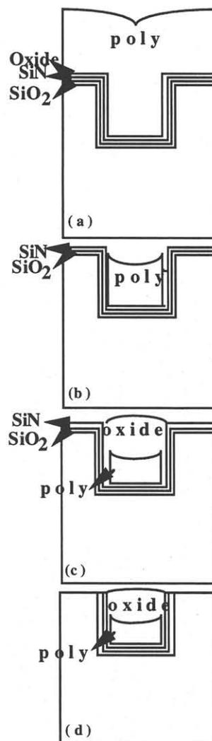
Fig. 1 The schematic process sequence of polysilicon-filled shallow trenches.
