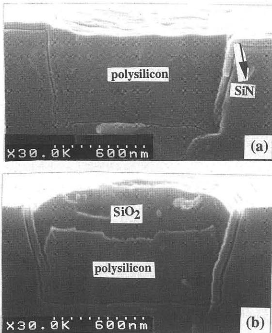
Fig. 3 The SEM micrographs (a) polysilicon-filled shallow trenches after a CMP process (b) polysilicon-filled shallow trenches after a local oxidation of polysilicon and the pad oxide/SiN layer stripped.
