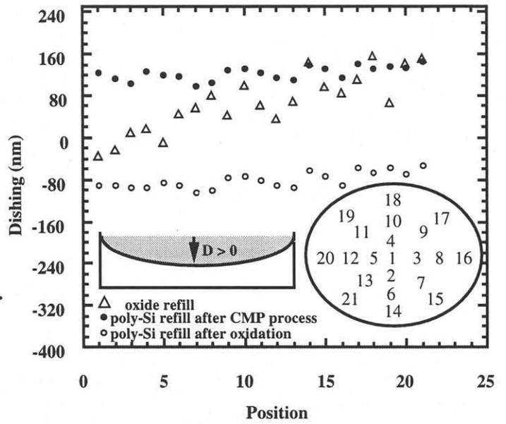
Fig. 5 The dishing distribution for 100-μm wide field regions across 6-inch diameter wafers..
