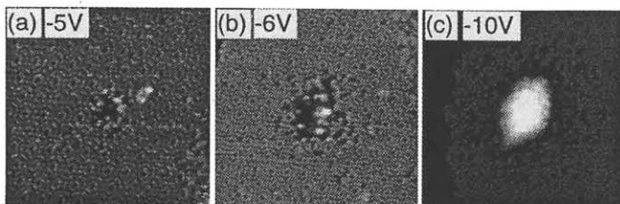
Fig. 2. Magnified STM images of the sample surfaces where voltages were applied: (a) -5 V for 5s, (b) -6 V for 5 s, and (c) -10 V for 55 s.
