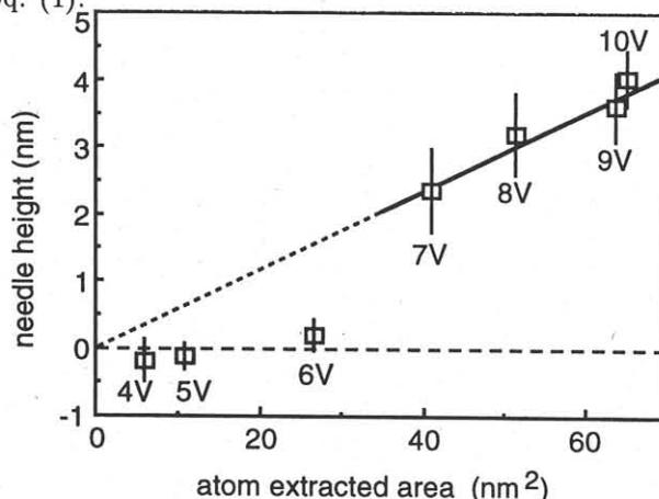
Fig. 4. The correlation between the atom extracted area and the nano-needle height.
