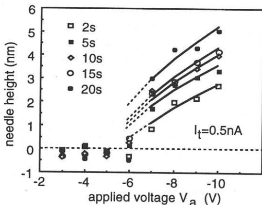
Fig. 1. The voltage dependence of nano-needle growth height for various duration times of applied voltage.
