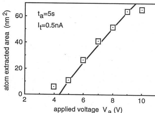
Fig. 3. The voltage dependence of the Si extracted area. The solid line shows the fitting curve by the Eq. (1).
