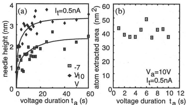
Fig. 5. The time dependence of (a) the nano-needle growth height and (b) the atom extracted area using positive tip voltages.
