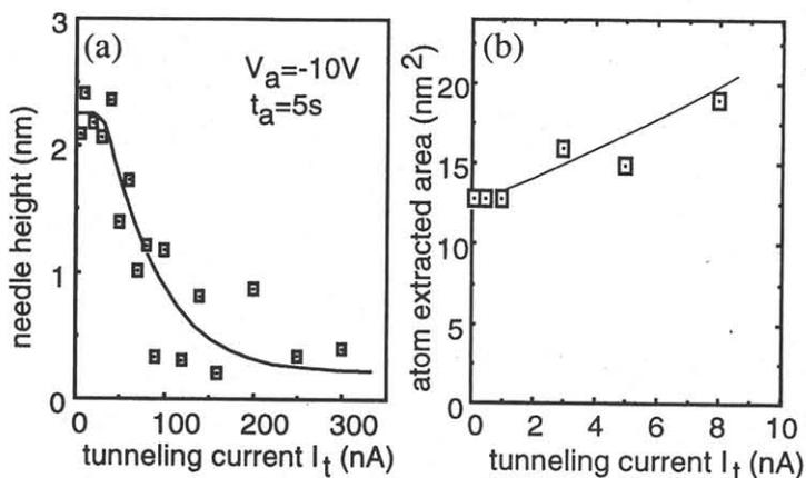
Fig. 6. The current dependence of (a) the nano-needle growth height and (b) the atom extracted area using positive tip voltages.
