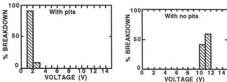
Figure 5. Comparison of gate oxide breakdowns for  $3.6 \times 10^{-3}$  cm<sup>2</sup> capacitors built on SIMOX with a high level of pitting defects and SIMOX wafers with a low level of pitting defects.
