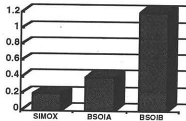
Fig. 3. Plot of generation lifetime in μSec for different SOI substrates.
