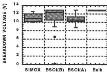
Fig.4 Capacitors showing the difference in BV for those on bulk and on SOI.
