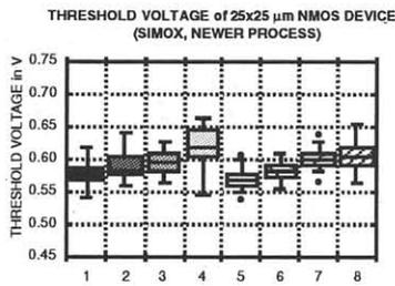
Fig. 2 Comparison of V<sub>t</sub> on several lots of SIMOX wafers.
