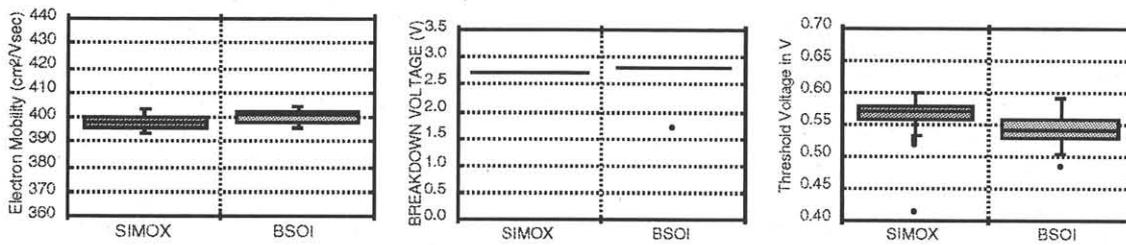
FIG. 1. Electron mobility, BVDSS and V<sub>t</sub> for devices in a split lot of SIMOX and BSOI showing no significant difference with material type.
