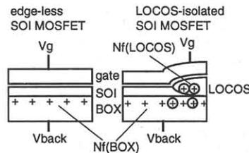
Fig. 6 Schematic diagram of edgeless and LOCOS-isolated SOI MOSFET's. By measuring of both devices, each fixed charges of  $N_f(\text{BOX})$  and  $N_f(\text{LOCOS})$  is able to be estimated.
