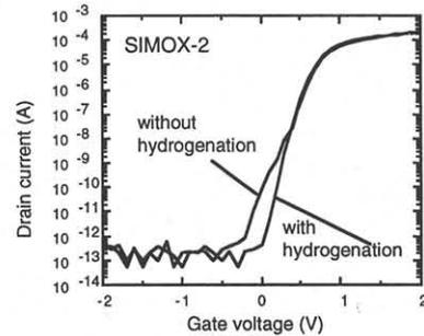
Fig.10 Measured Id-Vback characteristics of LOCOS-isolated SOI MOSFET's with and without hydrogenation. L/W=1.0  $\mu$  m/10  $\mu$  m
