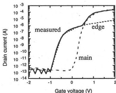
Fig.1  $I_d$ - $V_g$  characteristic of LOCOS-isolated SOI MOSFET. Measured current is consisted from the currents of the main-transistor and the edge transistor.
