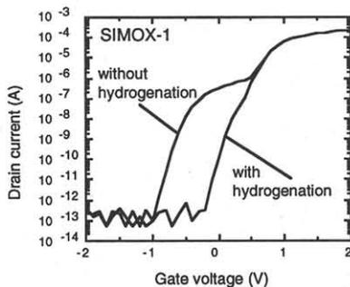
Fig.4 The comparison of measured Id-Vg characteristics in LOCOS-isolated SOI MOSFET's with and without hydrogenation.  $L/W=1.0 \mu\text{m}/10 \mu\text{m}$
