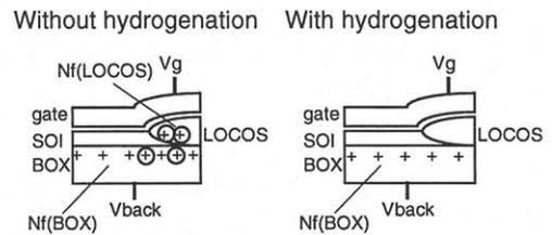
Fig.9 Schematic diagram of LOCOS-isolated SOI MOSFET's with and without hydrogenation. Nf(LOCOS) is reduced by hydrogenation.
