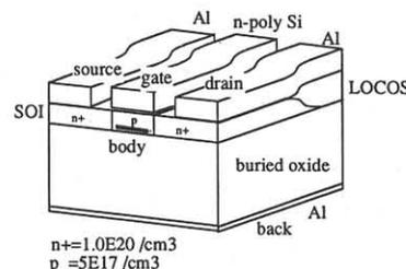
Fig.2 Schematic diagram of an SOI MOSFET analyzed by the 3-D simulation.
