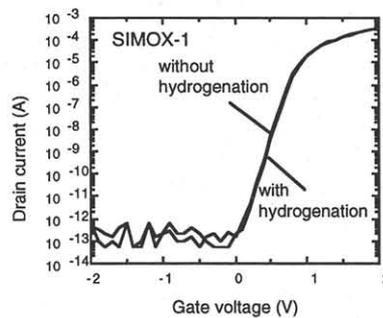
Fig.5 The comparison of measured Id-Vg characteristics in edgeless SOI MOSFET's with and without hydrogenation.  $L/W=1.0 \mu\text{m}/4.0 \mu\text{m}$ ,  $V_f(\text{body bias})=0\text{V}$ .
