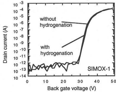
Fig.7 The comparison of measured Id-Vback characteristics in edgeless SOI MOSFET's with and without hydrogenation. L/W=1.0  $\mu$  m/4.0  $\mu$  m
