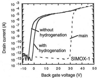
Fig.8 The comparison of measured Id-Vback characteristics in LOCOS-isolated SOI MOSFET's with and without hydrogenation. L/W=1.0  $\mu$  m/10  $\mu$  m
