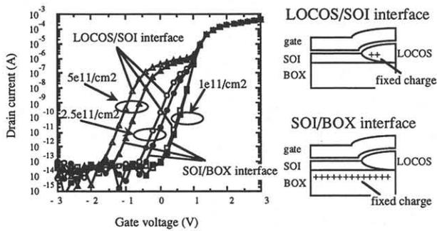
Fig.3 Simulated Id-Vg characteristics in LOCOS-isolated SOI MOSFET. Fixed charge is set in LOCOS/SOI or SOI/BOX interfaces.  $L=0.5 \mu\text{m}$
