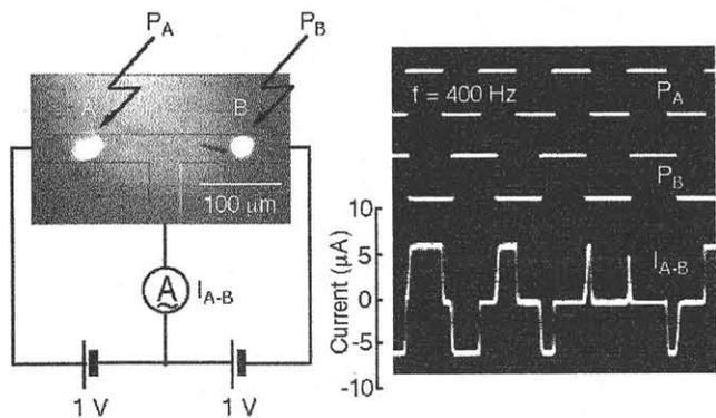
Fig. 4 Optical circuit for subtraction using two PCPTs, (a) where a chopped laser beam with a frequency of 400 Hz and that with a little different frequency are irradiated onto two point contacts, respectively. (b) shows the experimental result, where  $P_A$  and  $P_B$  correspond to the change of the laser power of the two laser beams and the lowest profile  $I_{A-B}$  is AC current measured by the ammeter shown in (a).
