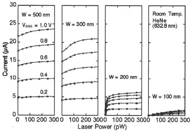
Fig. 1 Drain current profiles of the point contacts with various widths as a function of HeNe laser power at room temperature, where the bias voltage applied between the source and the drain was changed from 0.2 to 1.0 V with a step of 0.2 V as indicated at the right side of each curve for the 500-nm sample.
