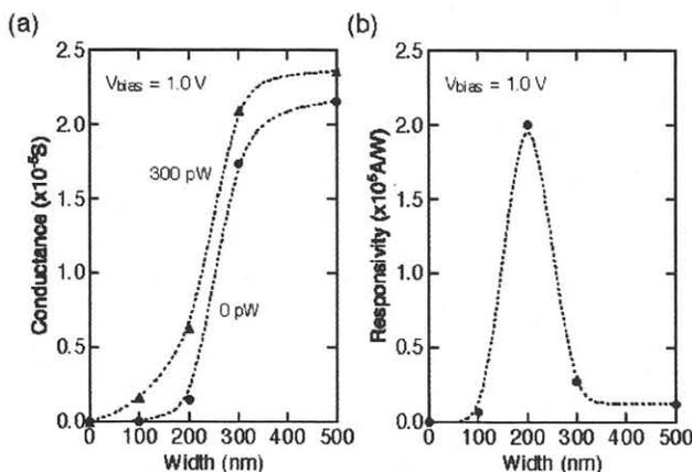
Fig. 2 Conductance at laser powers of 0 and 300 pW and a bias voltage of 1 V. (a) Responsivity at 5 pW and 1 V as a function of width of point contacts. (b)
