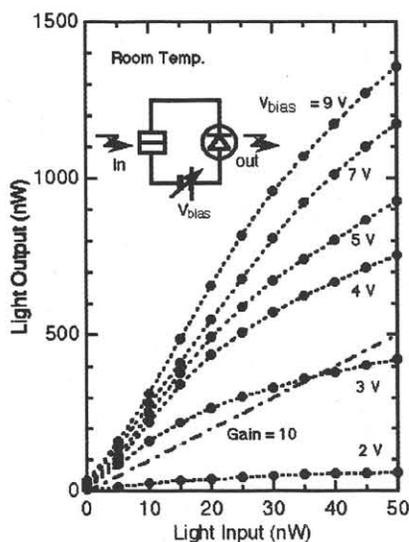
Fig. 5 Output profile of the optical amplifier using a point contact phototransistor and a light emitting diode as a function of input light power at room temperature. A inset shows the circuit, and a chain line indicates a gain of 10.
