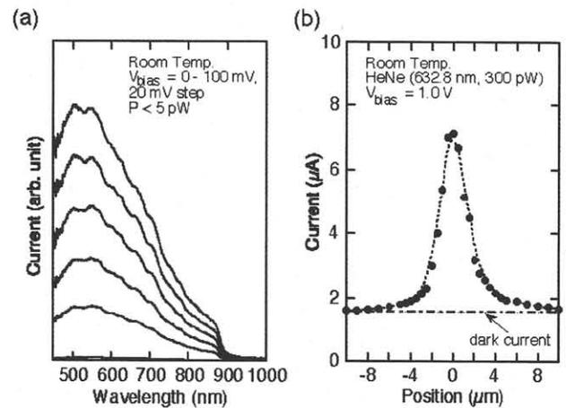
Fig. 3 Current through the point contact with a width of 200 nm measured by a lock-in amplifier as a function of wavelength of the spectral-resolved incident light, where power of the light was less than 5 pW, the light diameter on the sample was set less than 1  $\mu\text{m}$ , and the light was irradiated just on the point contact. (a) Current through the point contact measured in changing the position illuminated by the laser beam. (b)
