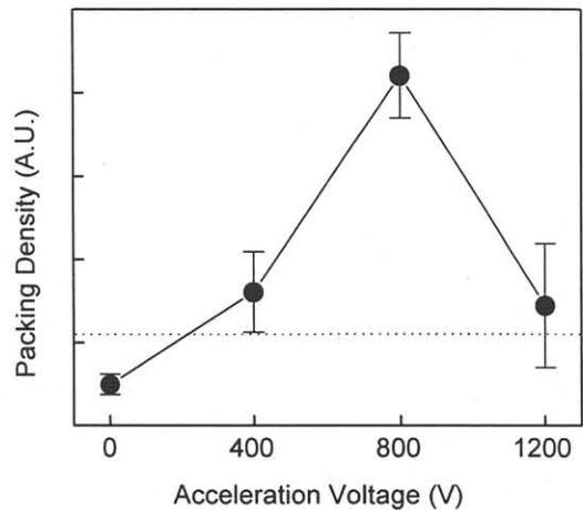
Fig. 1. Packing Density Variation with Acceleration Voltage.
