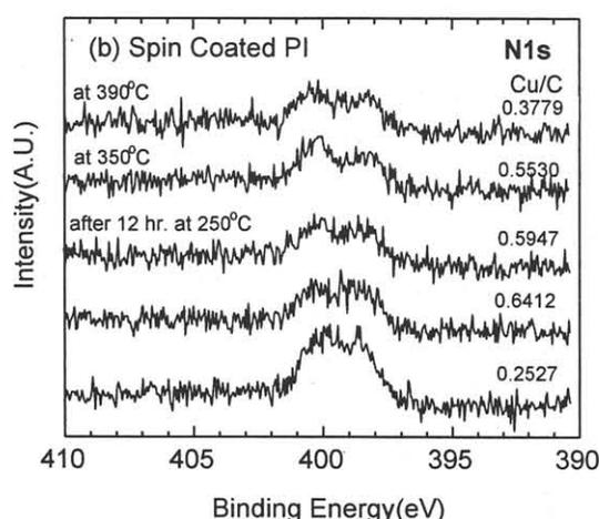
Fig. 3. N 1s core-level spectra measured during *in-situ* formation of the Cu/PI interface as a function of Cu coverage at 250°C for (a) ICB PI and (b) Spin Coated PI
