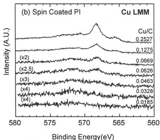
Fig. 2. Cu LMM X-ray induced Auger peaks measured during *in-situ* formation of the Cu/PI interface as a function of Cu coverage at 250°C for (a) ICB PI and (b) Spin Coated PI
