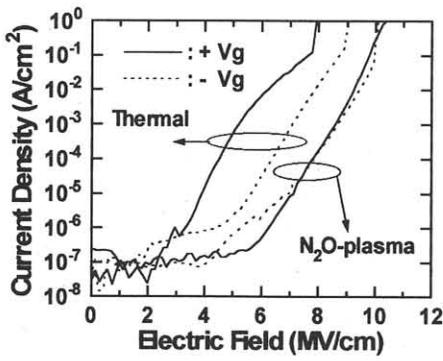
Fig. 1 Current density versus electric field plots for thermal oxide and N<sub>2</sub>O-plasma oxide on poly-Si (deposited in *in-situ* doping followed by thermal annealing for crystallization).
