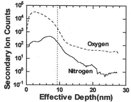
Fig. 6 SIMS depth profiles of N<sub>2</sub>O-plasma polyoxide. The vertical dotted line indicates Si/SiO<sub>2</sub> interface.
