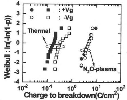
Fig. 5 Weibull plots of charge-to-breakdown of capacitors with thermal polyoxide and N<sub>2</sub>O-plasma polyoxide, measured at current density of 10mA/cm<sup>2</sup>.
