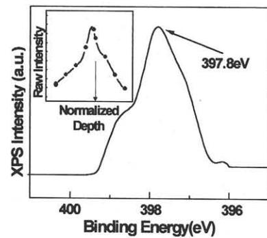
Fig. 7 XPS N(1s) intensity of N<sub>2</sub>O-plasma oxide at the interface. Inset : depth profile of N(1s) intensity.
