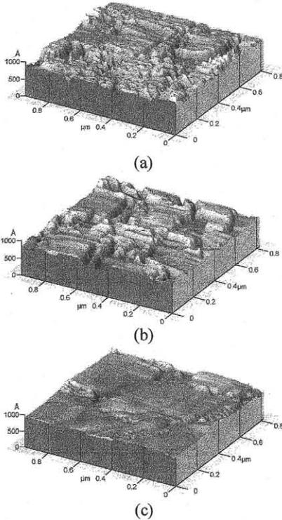
Fig. 3 AFM images of surface of poly-Si (a) without oxidation, (b) after thermal oxidation, and (c) after N<sub>2</sub>O-plasma oxidation. The corresponding rms roughness are 6.4nm, 9.6nm, and 4.6nm respectively.
