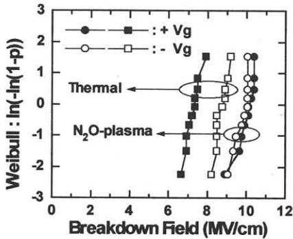
Fig. 2 Cumulative weibull distribution of breakdown field for thermal polyoxide and N<sub>2</sub>O-plasma polyoxide
