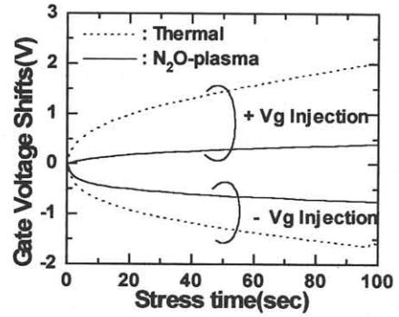
Fig. 4 Gate voltage shifts during constant current stressing with 1mA/cm<sup>2</sup> for thermal polyoxide and 10mA/cm<sup>2</sup> for N<sub>2</sub>O-plasma polyoxide.
