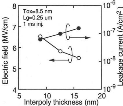
Fig. 10 Electric field and leakage current dependence on the interpoly thickness
