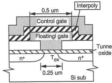
Fig. 2 Schematic diagram of 0.25- $\mu$ m AND type memory cell
