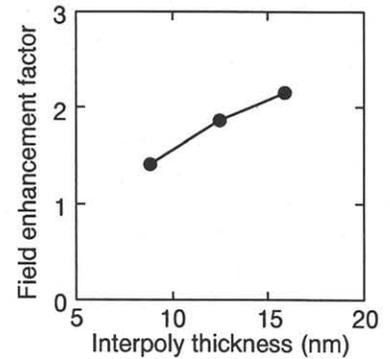
Fig. 9 Dependence of electric field enhancement on the interpoly thickness
