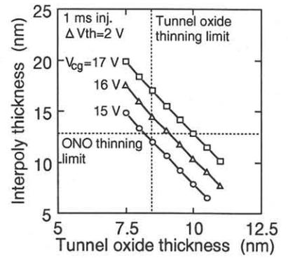
Fig. 3 Interpoly dielectric film thickness vs tunnel oxide thickness
