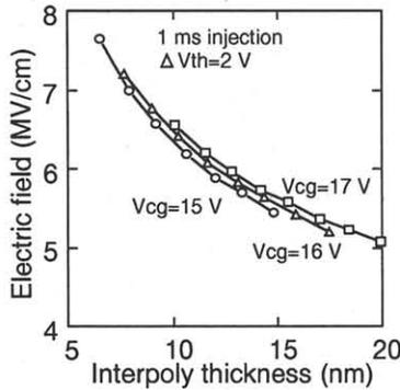
Fig. 4 Electric field across interpoly dielectric films after 1 ms injection
