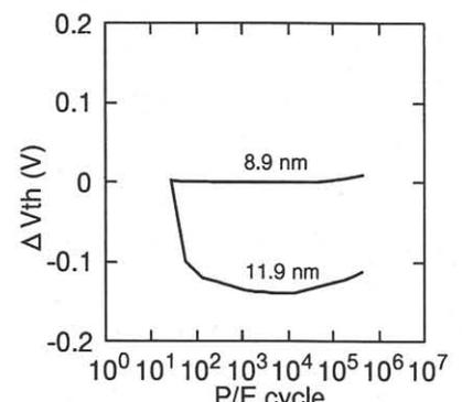
Fig. 12 Calculated  $V_{th}$  shift of the memory cell caused by charge trapping in the interpoly
