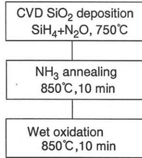
Fig. 5 Process flow for  $\text{NH}_3$ -annealed CVD  $\text{SiO}_2$  single-layer interpoly
