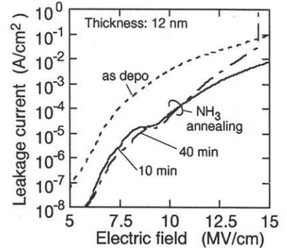
Fig. 6 J-E characteristics of  $\text{NH}_3$ -annealed CVD  $\text{SiO}_2$  single-layer films
