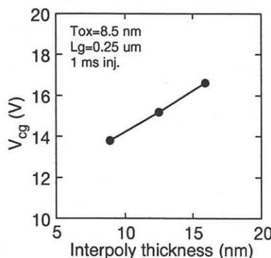
Fig. 11 Programming voltage reduction by thinning the interpoly thickness
