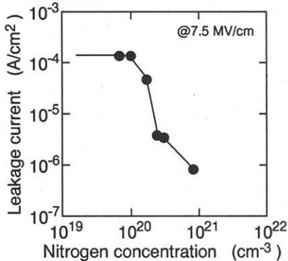
Fig. 7 Leakage current dependence on nitrogen concentration in the  $\text{SiO}_2$  films
