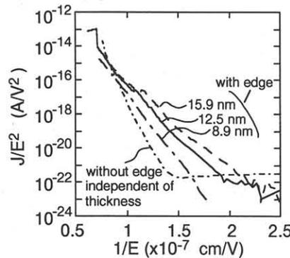
Fig. 8 F-N plots of  $\text{NH}_3$ -annealed CVD  $\text{SiO}_2$  single-layer films
